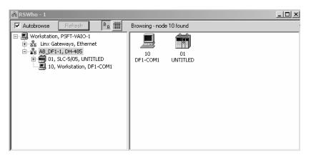
3 Notice how the DF1 driver is opened, and the driver is looking for node 1 (an SLC processor). If the network is being browsed, then you will not be able to stop this driver. To stop the driver your RSWho screen should look like this:
