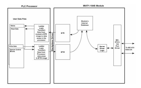
As shown in the diagram above, all data transferred between the module and the processor over the backplane is through the BTR and BTW blocks. Ladder logic must be written in the PLC processor to interface the block data with user data files. All data used by the module is stored in its internal database. The following illustration shows the layout of the database:
