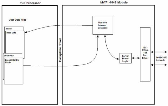
The configuration information for the module determines the size of the read and write data areas and the locations of these data sets in the module's internal database. Therefore, to use this interface, just set up the files required by the module. The following table lists the files required for the side-connect interface.
