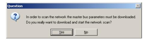
When the download is completed, the *PROFIBUS Master Configuration* window will initialize the Master to operate as a *Class1/Class 2 Master*. In this mode it is possible to initialize the Master even if the database does not contain any slaves. After successful initialization, the *PROFIBUS Master Configuration* window will
