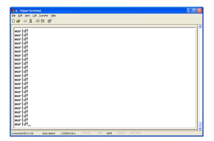
14 You can view how the stream of data is accepted by the LDM module by untoggling the Serial\_App\_Sample\_WriteTrigger and typing a string of characters on the console.
