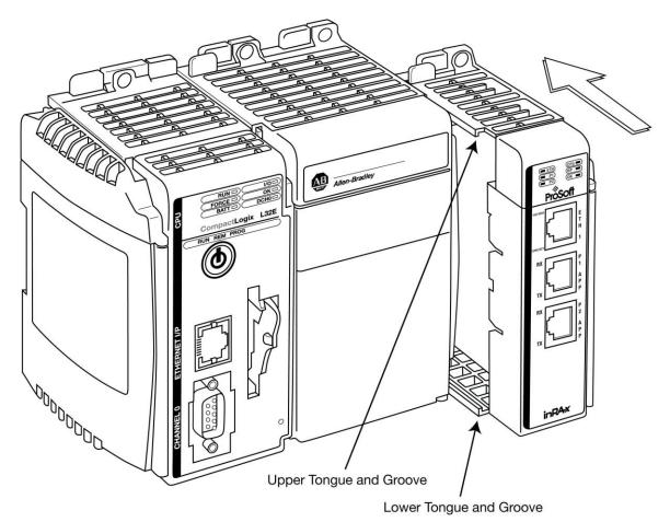
2 Move the module back along the tongue-and-groove slots until the bus connectors on the MVI69E module and the adjacent module line up with each other. Push the module's bus lever back slightly to clear the positioning tab and move it firmly to the left until it clicks. Ensure that it is locked firmly into place.
