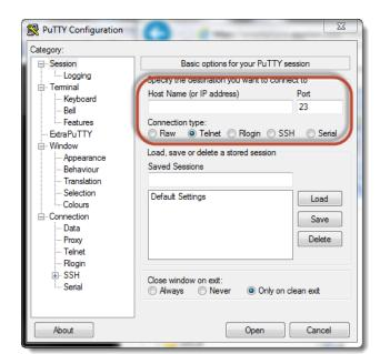
3 Use a program such as PuTTY to Telnet into the module.
