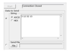
Click **START** to transmit the data from the computer into the module and backplane. It is then updated in RSLogix 5000 with the appropriate number associations.
