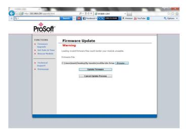
5 Click **UPDATE FIRMWARE** and wait for the module to reboot. During rebooting, the module expands the compressed file and runs the install script to move the component files to their final destination.
