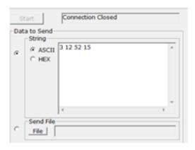
Select **START** to transmit the data from the computer into the module and backplane. It is then updated in RSlogix5000 with the appropriate number associations.
