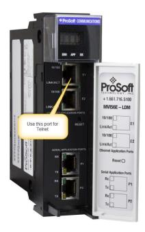
Connect an Ethernet RJ45 cable to the E1 port of the module and the other end to the network switch.
