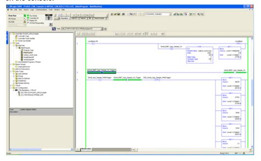
**16** The letter 'h' appears in the location *Local:1:I.Data*. Make sure that the Style column in the ControlLogix is set to *ASCII*.
