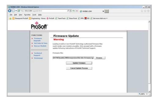
5 Click on the **UPDATE FIRMWARE** button and wait for the module to reboot. During reboot, the compressed file is un-"tar" ed and the install script is run to move the component files to their final destination.
