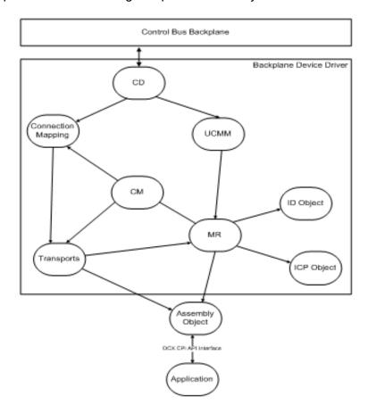
All data exchange between the application and the backplane occurs through the Assembly Object, using functions provided by the CIP API. The API includes functions to register or unregister the object, accept or deny Class 1 schedule connections requests, access scheduled connection data, and service unscheduled messages.
