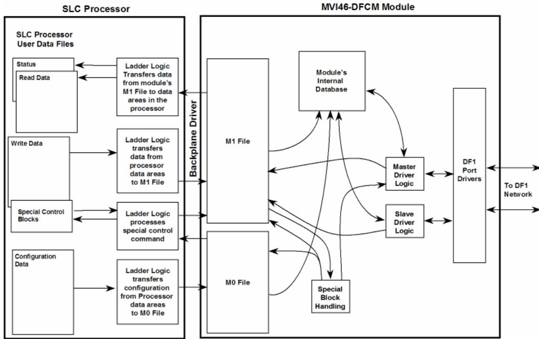
All data transferred between the module and the processor over the backplane is through the M0 and M1 files. Ladder logic must be written in the SLC processor to interface the M-file data with data defined in the user-defined data files in the SLC. All data used by the module is stored in its internal database. The following illustration shows the layout of the database:
