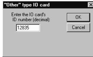
Enter the module I/O card ID number as 12835, and then click OK. Double-click the mouse on the module just added to the rack. Fill in the dialog box presented as shown below:
