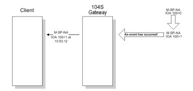
The gateway supports a buffer queue of 99 events per data type. When the queue is full, the gateway will delete the oldest event in the queue, replacing it with the newest event received for that data type.
