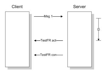
If the gateway does not receive the TESTFR.con message within a certain amount of time, it will timeout and close the connection. You can configure the timeout period using the following parameter:
