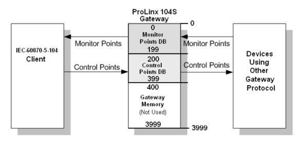
In this example, all monitor points are located between database addresses 0 and 199, and all control points are located between address 200 and 399.
