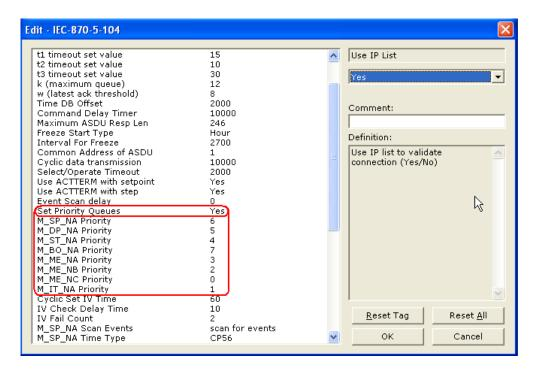
The Set Priority Queues parameter must be enabled for this feature to be used. Each of the ASDUs affected by this feature must be assigned a unique priority index from 0 to 7. Events of the ASDU with a priority of 0 will always be reported before any others when they are present.
