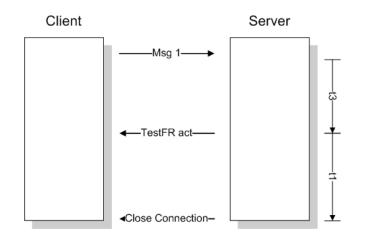
When closing the connection, the gateway can be configured to clear all the messages in its queue. The following parameter is used to implement this task:
