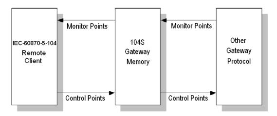
All points must be configured in the correct location in the 104S database in order to be properly updated by the other gateway protocol by configuring the control points and monitor points in separate areas of the 104S database. The following illustration shows an example configuration:
