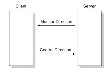
The points that are typically transferred from a server to a Client are also known as **Monitor Points** (or Monitor Information Objects). The points that are typically transferred from a Client to a server are also known as **Control Points** (or Command Information Objects).
