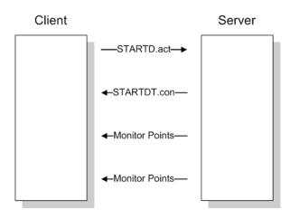
In some circumstances the client unit may not support STARTDT and STOPDT messages. The gateway may also be tested with simulator software that does not support these features. For these situations, you may want to disable the STARTDT and STOPDT features using the following parameter:
