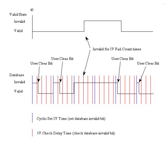
If a database bit address (1 to 64000) is present, the application may consider the point with an invalid flag if the previous logic checks the IV bit as 1 during consecutive IV Check Delay scans. The IV bits would have to be reset to 0 to set the point to valid state.
