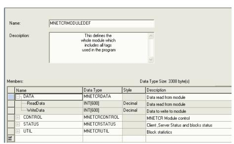
Notice that these UDTs are the data types used to declare the MNETCR.DATA.ReadData and MNETCR.DATA.WriteData controller tag arrays.
