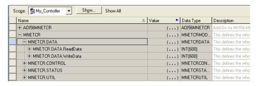
Each controller tag in the Add-On Instruction is commented in the *Description* column. Notice that the *Data Type* column displays the data types used to declare each controller tag, controller tag array or controller tag structure. Individual controller tags are declared with basic data types, such as INT and BOOL. Controller tag arrays are declared with arrays of basic data types. Controller tag structures are declared with user-defined data types (UDTs).
