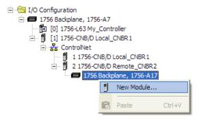
2 This action opens the *Select Module* dialog box. Expand the **OTHER** node, and then select **1756-MODULE** (**GENERIC 1756 MODULE**).
