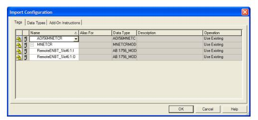
**10** Associate the I/O connection variables to the correct module. The default values are RemoteENBT Slot6:1:I and RemoteENBT Slot6:1:O, so these require change.
