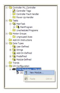
2 Expand the Communications module selections and then select the Ethernet Bridge module that matches your hardware. This example uses a 1756-ENBT/A module.
