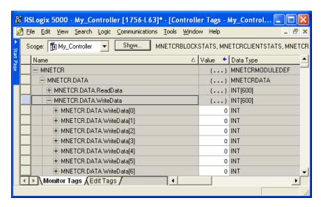
The *WriteData* array is related to the contents of the Write Data area of the module's internal database. To view the actual registers in the module's internal database, access the database display from *ProSoft Configuration Builder's Diagnostics* menu. For more information, see the section on *PCB* Diagnostics (page 78).
