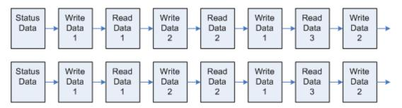
This sequence will continue until interrupted by other special function blocks sent by the processor, by a command request from a node on the Modbus network, or by operator control through the module's Configuration/Debug port.
