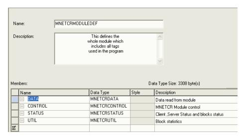
Click the **[+]** signs to expand the UDT structures and view lower-level UDTs. For example, if you expand *MNETCR.DATA*, you will see that it contains two UDTs, *ReadData* and *WriteData*. Both of these are 600-element integer arrays by default.
