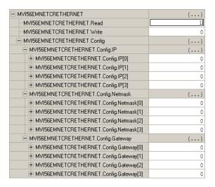
The bit will be automatically reset and the current Ethernet settings will be copied to **MVI56EMNETCRETHERNET** controller tag as follows.
