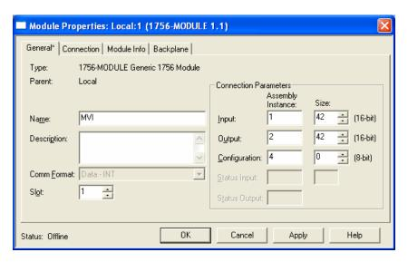
In the **SLOT** field, use the up and down arrows on the right side of the field to select the slot number where the module will reside in the rack, and then click **OK**.
