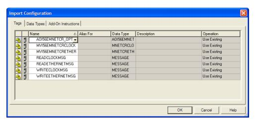
The Add-On Instruction will now be visible in the ladder logic. Observe that the procedure has also imported data types and controller tags associated to the Add-On Instruction.
