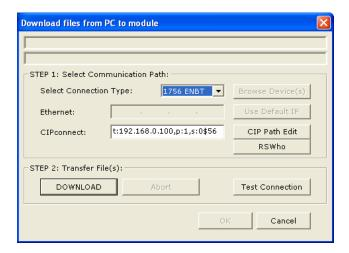
**4** Click **RSWHO** to display modules on the network. The MVI56E-MNETCR module will automatically be identified on the network.
