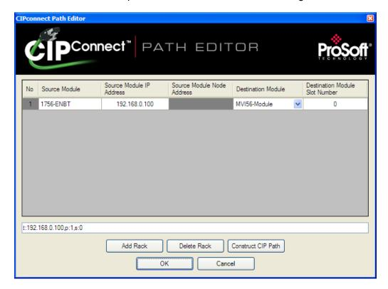
The CIPconnect Path Editor allows you to define the path between the PC and the MVI56E-MNETCR module. The first connection from the PC is always a 1756-ENBT (Ethernet/IP) module.
