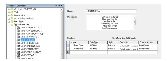
2 Edit the *ReadData* array size to match or exceed the value of the *Read Register Count* parameter in PCB.
