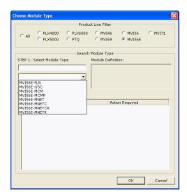
In the *Product Line Filter* area of the dialog box, select **MVI56E**. In the *Select Module Type* dropdown list, select **MVI56E-MNETCR**, and then click **OK** to save your settings and return to the *ProSoft Configuration Builder* window.
