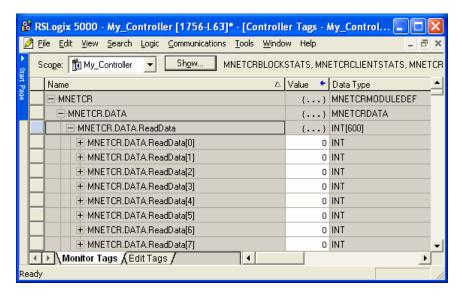
The *ReadData* array is related to the contents of the Read Data area of the module's internal database. To view the actual registers in the module's internal database, access the database display from *ProSoft Configuration Builder's Diagnostics* menu. For more information, see the section on *PCB* Diagnostics (page 78).
