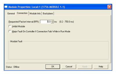
**4 Save the module.** Click **OK** to dismiss the dialog box. The *Controller Organization* window now displays the module's presence.
