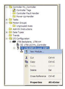
6 Repeat steps 2 and 3 to add the second EtherNet/IP module to the remote rack.
