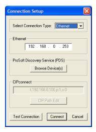
You can also use CIPconnect<sup>®</sup> to connect to the module through a 1756-ENBT card. Refer to Using CIPconnect to Connect to the Module (page 54) for information on how to construct a CIP path.
