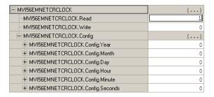
The bit will be automatically reset and the current clock value will be copied to **MVI56EMNETCRCLOCK.CONFIG** controller tag as follows.
