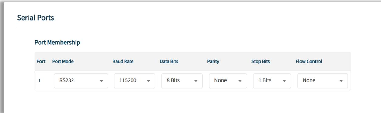
The screenshot shows the 'Serial Ports' configuration interface. Under the 'Port Membership' tab, a table displays the following settings for port 1:
