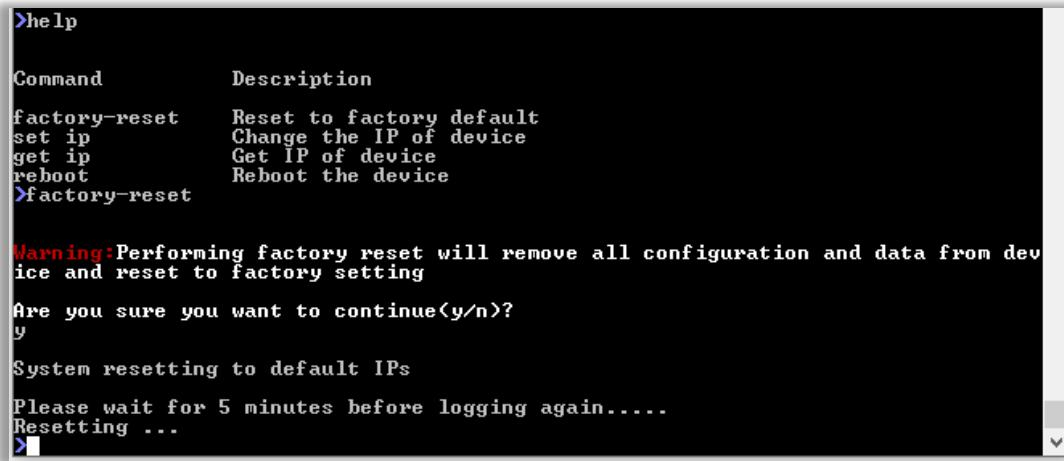
A terminal window showing the factory reset process. The user types 'factory-reset' and the system prompts for confirmation. The user types 'y' and the system begins the reset process, indicating a 5-minute wait before logging again.
