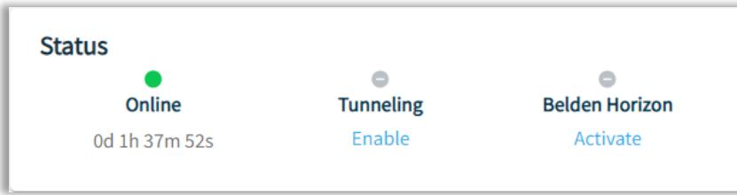
**Note:** If the ELX3 is already connected to a Belden Horizon Console account, the link states “**Deactivate**”.
