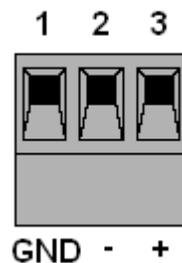
Left to right the pins on the power connector are chassis ground, negative voltage and positive voltage. Pin 1 is closest to the Ethernet connector.
