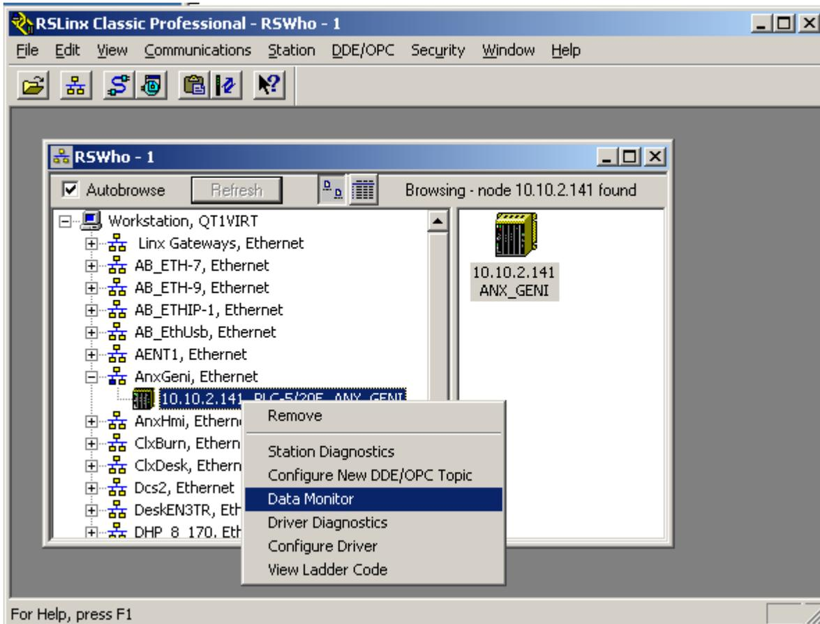
First create an Ethernet driver to communicate with the AN-X3.
