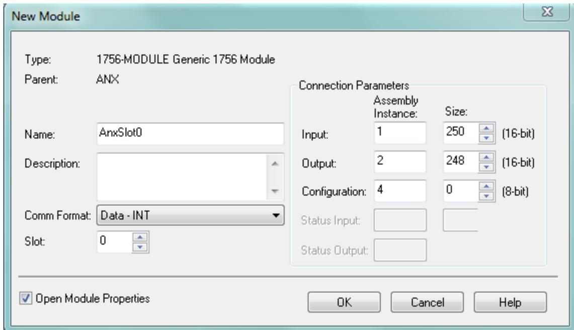
Set the parameters as shown. Set the Slot to 0 for the first connection, 1 for the second connection, and so on.
