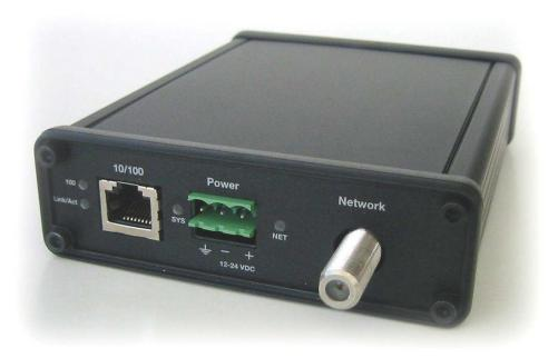
The AN-X3-MOD-MON allows an Ethernet/IP Client such as ControlLogix to monitor Modicon S908 RIO network I/O data.
