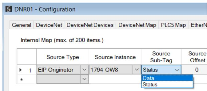
Figure 5.21 – IDS Copy – EtherNet/IP Originator Status
