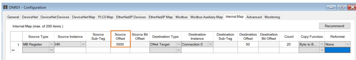
Figure 5.28 – Internal Mapping from Modbus Register to DeviceNet
