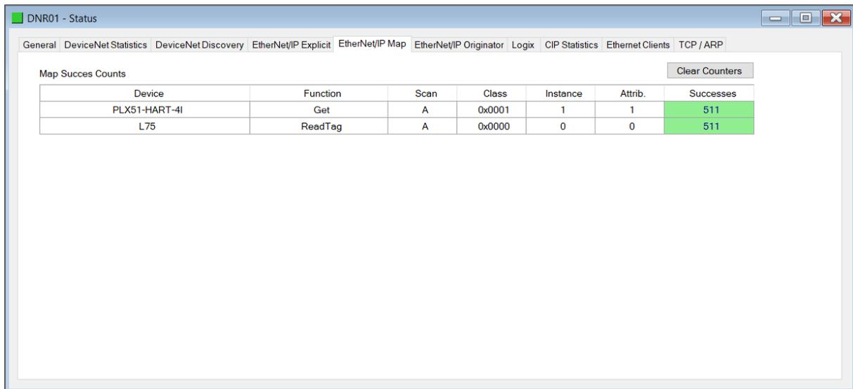
Figure 6.10 - Status monitoring – EtherNet/IP Map
