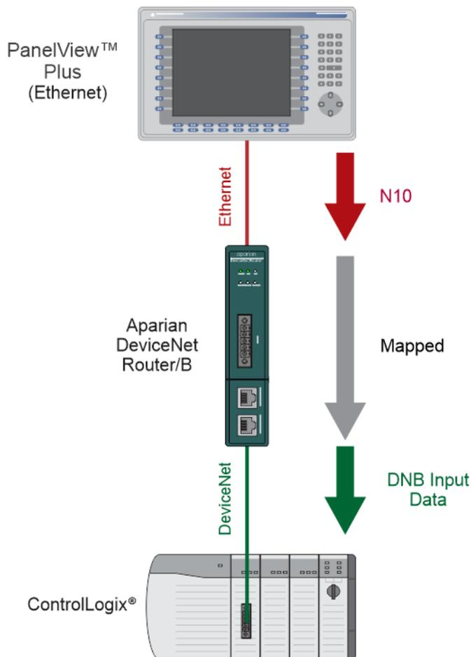
Figure 5.33 – PanelView writing Logix data over Cyclic DeviceNet
