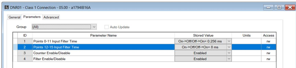
Figure 3.50 – DeviceNet Flex IO Parameter configuration
