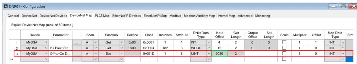
Figure 5.11 – Explicit Messaging – Set Function from IDS to DeviceNet device
