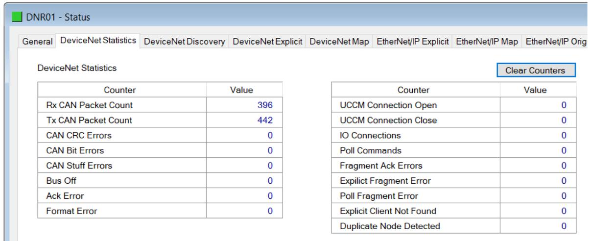
Figure 6.5 - Status monitoring – DeviceNet Statistics
