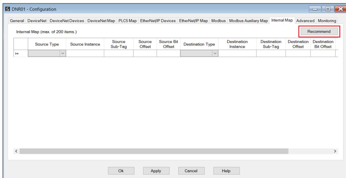
Figure 3.93 – Modbus Server – Internal Mapping Recommend
