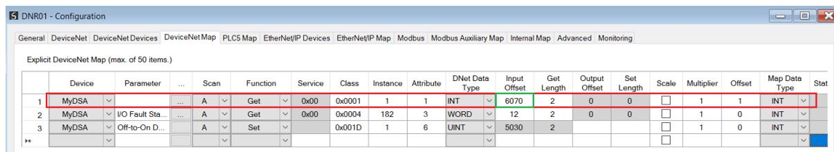
Figure 5.12 – Explicit Messaging – Get Function from DeviceNet device to IDS
