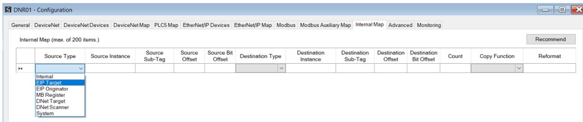
Figure 3.90 – IDS Copy – EtherNet/IP Target Source Type
