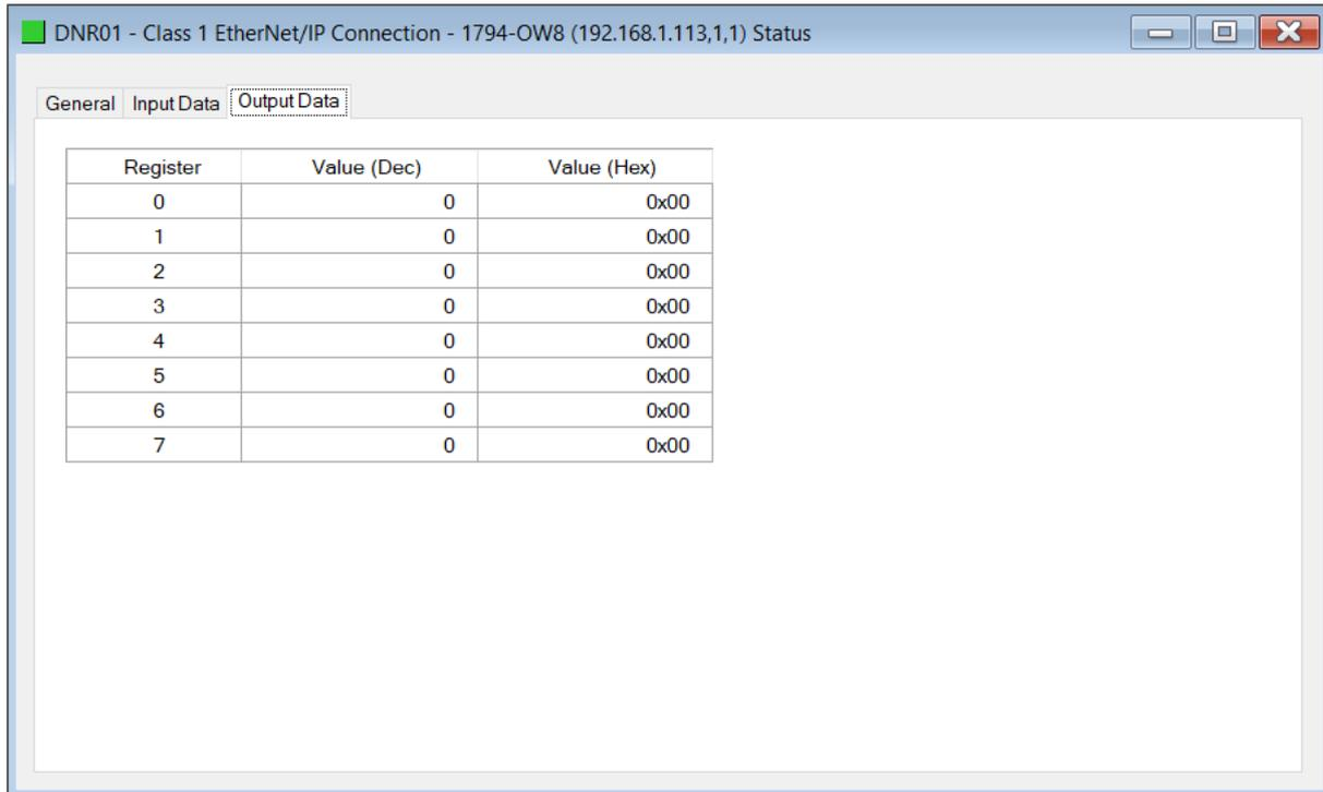
Figure 6.20 – EtherNet/IP Device Status – Output Data
