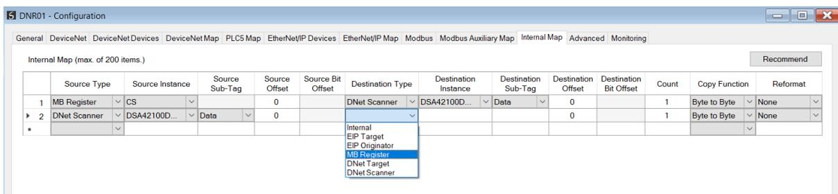
Figure 3.105 – IDS Copy - Modbus Destination Type
