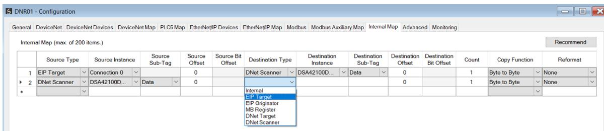
Figure 3.91 – IDS Copy – EtherNet/IP Target Destination Type
