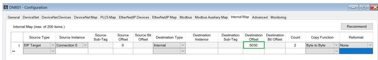
Figure 5.10 – Internal Mapping from EtherNet/IP to IDS
