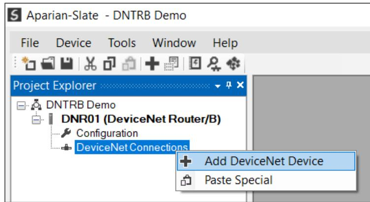
Figure 3.42 – Adding DeviceNet Cyclic IO Device Connection
