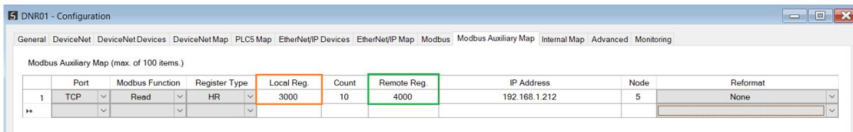
Figure 5.27 – Modbus Client Aux Mapping
