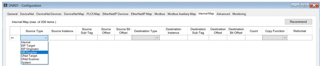
Figure 3.133 – IDS Copy - Modbus Source Type
