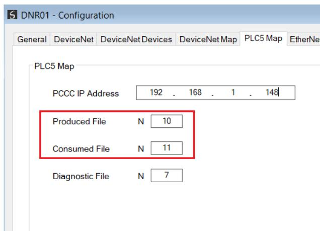
Figure 5.31 – PLC File configuration
