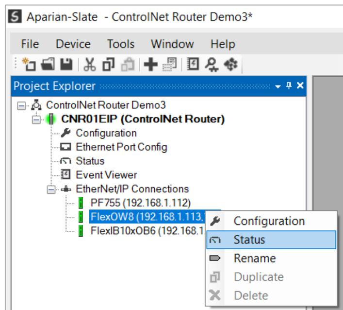
Figure 6.17 – EtherNet/IP Device Status – Status selection
