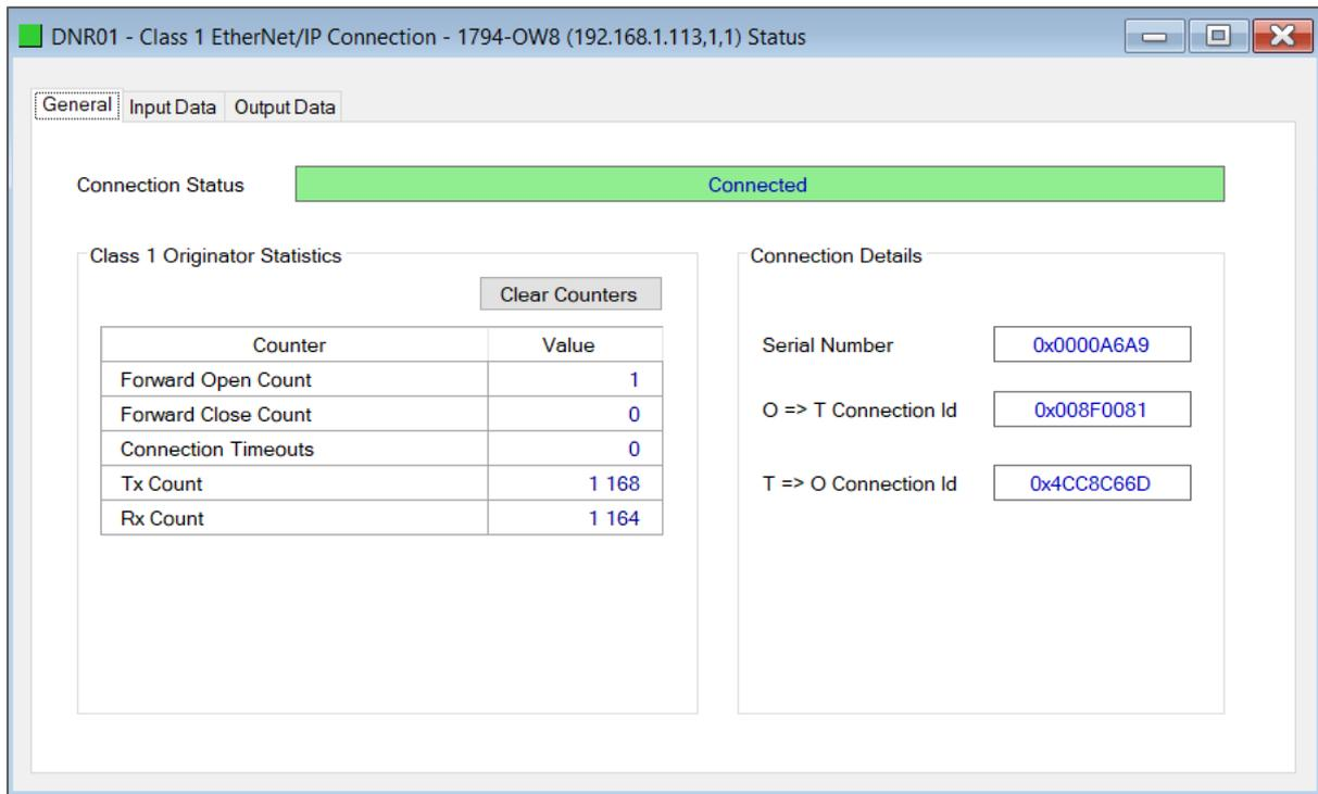
Figure 6.18 – EtherNet/IP Device Status – General Status
