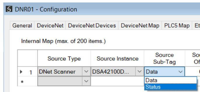
Figure 3.138 – IDS Copy – EtherNet/IP Originator Status
