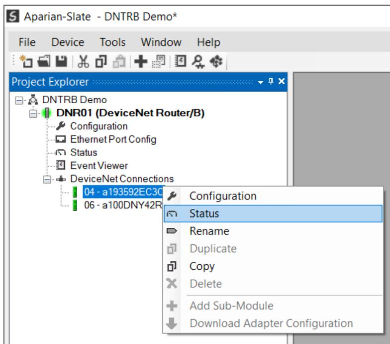
Figure 6.21 – DeviceNet Device Status – Status selection
