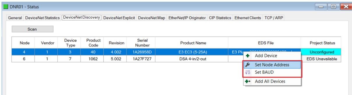
Figure 5.16 – DeviceNet Discovery – Set Node Address and BAUD
