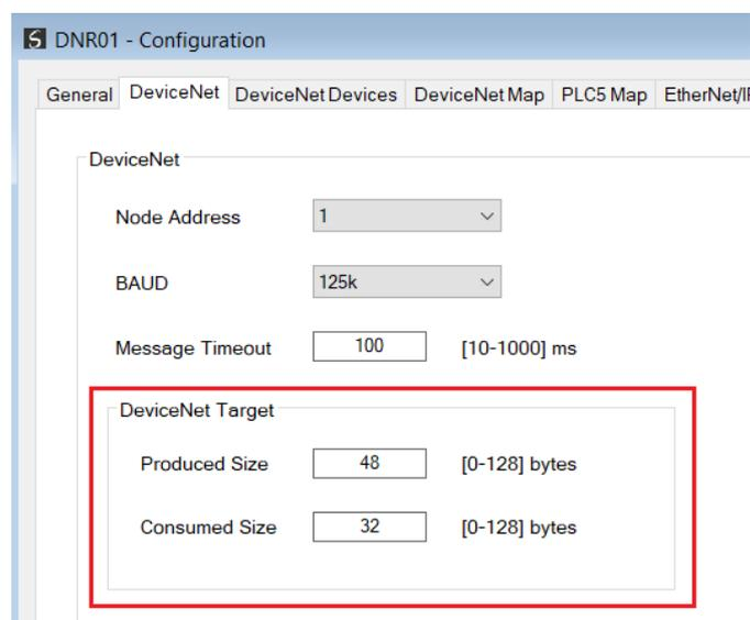
Figure 5.1 – DeviceNet Target Produce and Consume size
