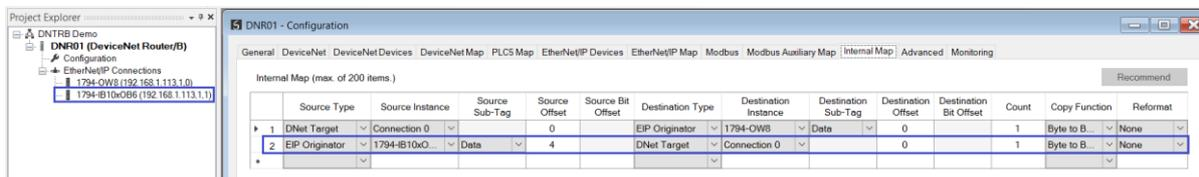
Figure 5.20 – Internal Mapping from EtherNet/IP Originator to DeviceNet
