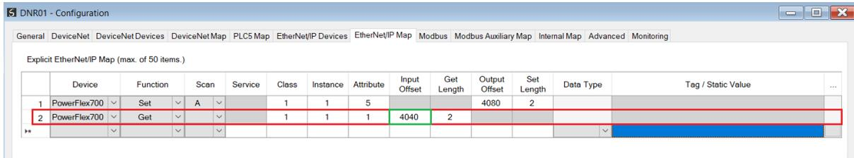
Figure 5.24 – Explicit Messaging – Get Function from EtherNet/IP device to IDS
