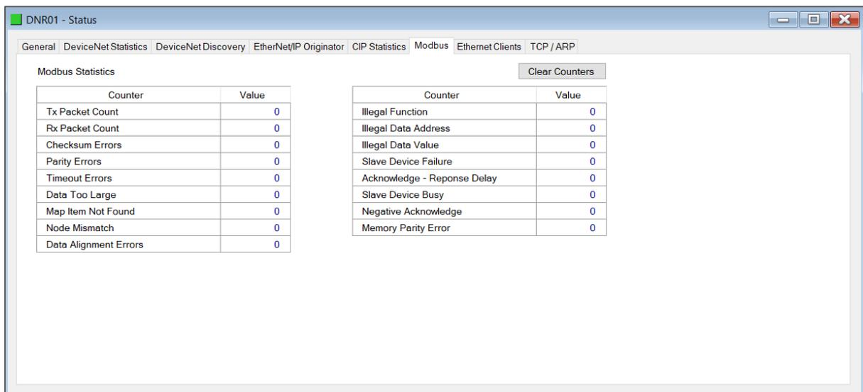
Figure 6.13. - Status monitoring – Modbus Statistics
