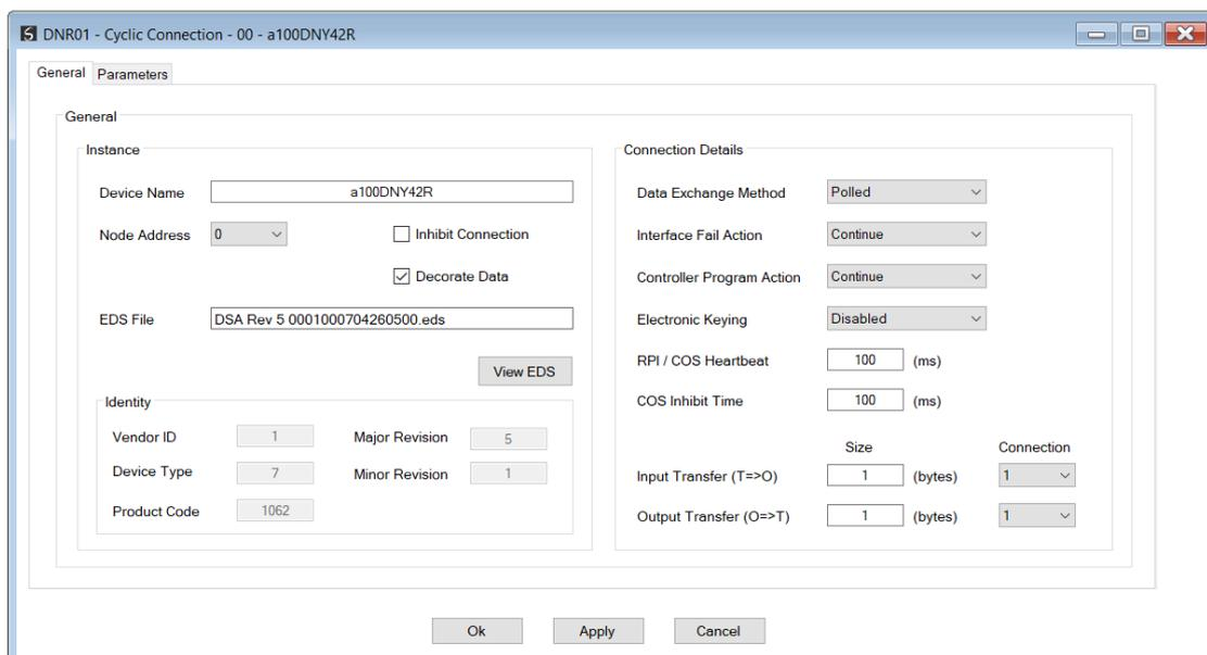
Figure 3.43 – IO Device Cyclic DeviceNet Connection Parameters
