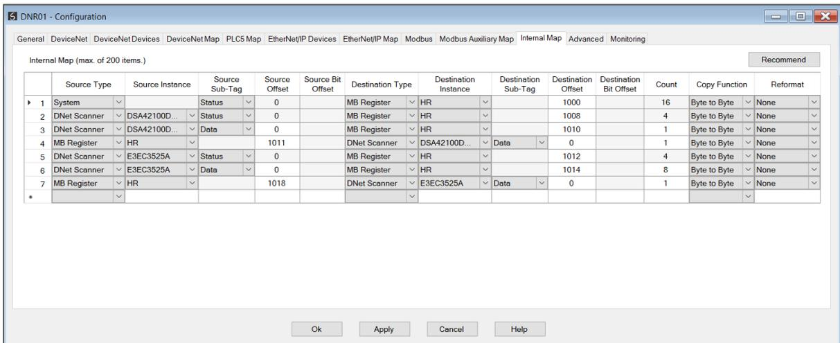
Figure 3.102 – Modbus Server – Internal Mapping Updated
