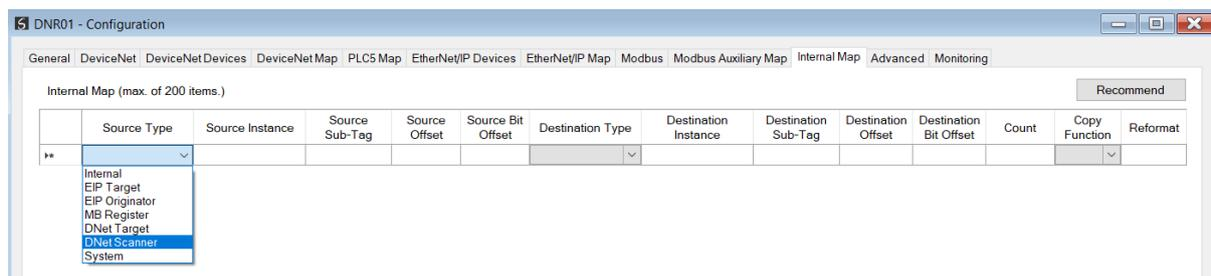
Figure 3.57 – IDS Copy – DeviceNet Scanner Source Type
