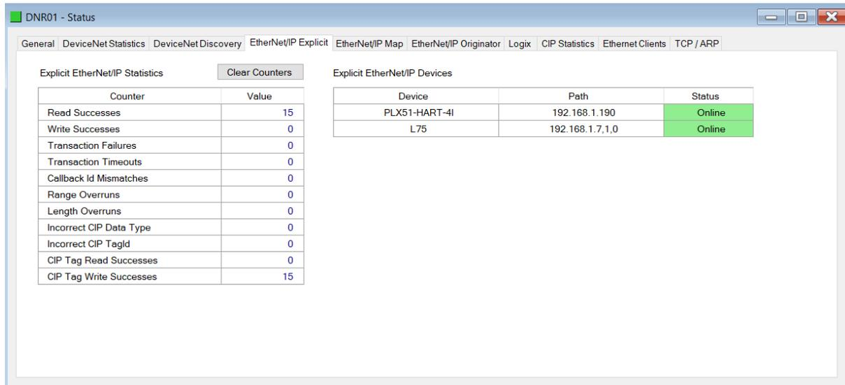
Figure 6.9 - Status monitoring – EtherNet/IP Explicit
