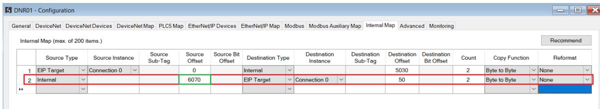
Figure 5.13 – Explicit Messaging – Internal Mapping from IDS to EtherNet/IP
