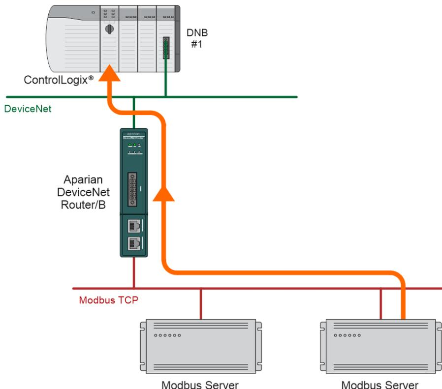
Figure 5.26 – Modbus Client to DeviceNet operation
