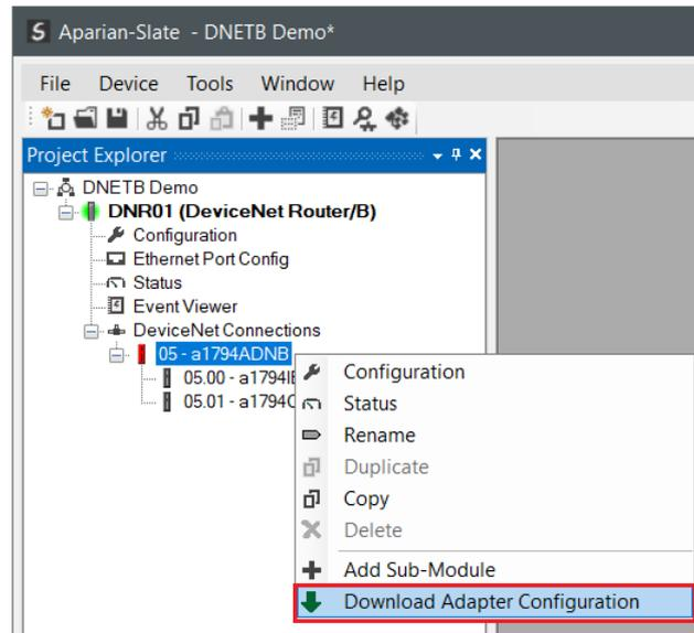
Figure 3.54 – DeviceNet Flex IO Adapter – Download Configuration
