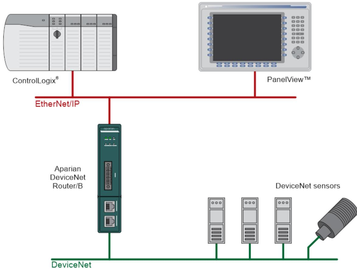
Figure 1.1. – Typical DeviceNet Scanner architecture using the DeviceNet Router/B
