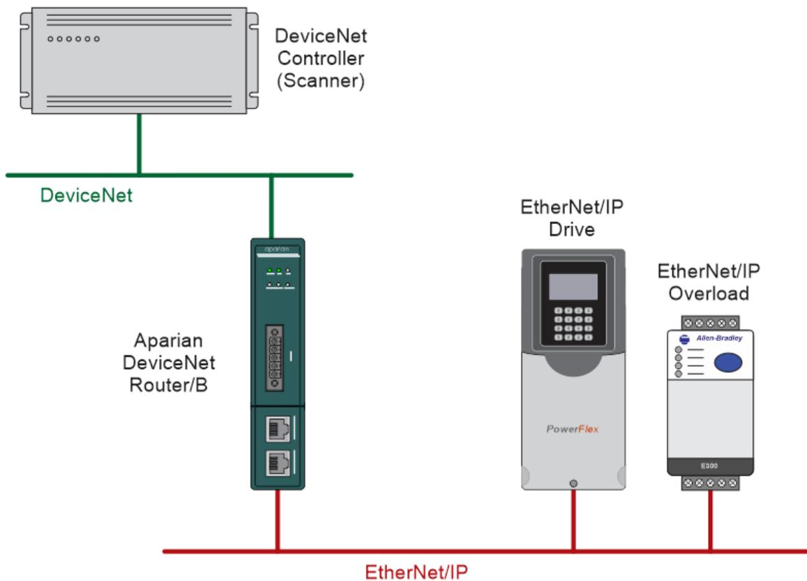
Figure 1.9. – EtherNet/IP Drive and Smart Overload operating as a DeviceNet Device
