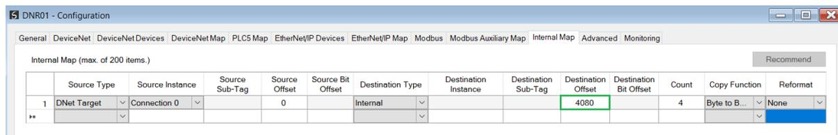
Figure 5.22 – Internal Mapping from DeviceNet to IDS
