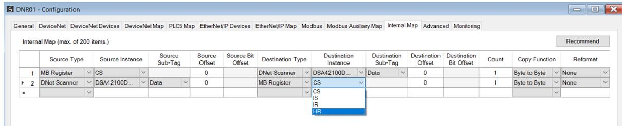
Figure 3.106 – IDS Copy - Modbus Destination Instance
