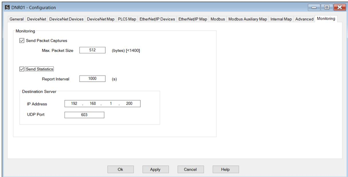
Figure 3.151 – Monitoring configuration
