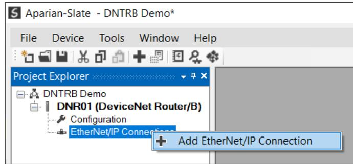
Figure 3.107 – Adding EtherNet/IP Class 1 Connection
