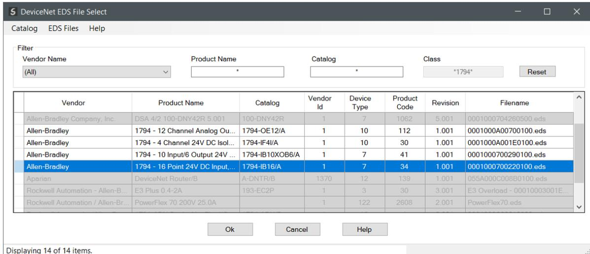
Figure 3.48 – Select the DeviceNet Flex IO Module
