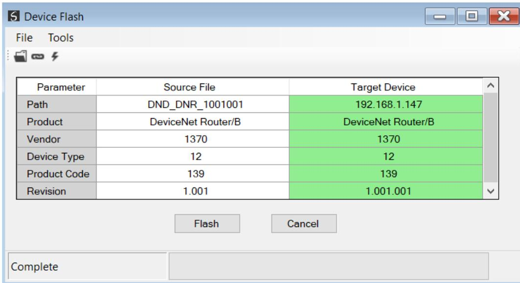
Figure 4.5 – Firmware update successfully completed.
