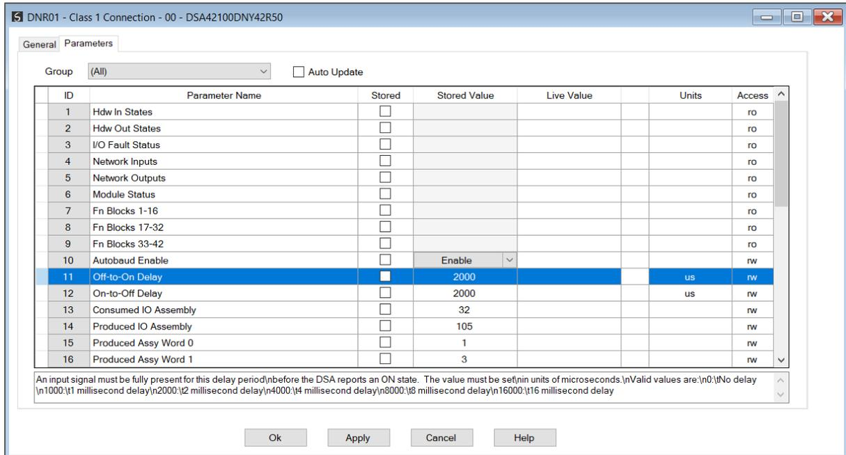
Figure 3.44 – IO Device Cyclic DeviceNet Parameters
