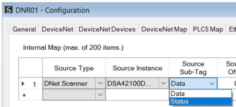
Figure 5.35 – IDS Copy – EtherNet/IP Originator Status
