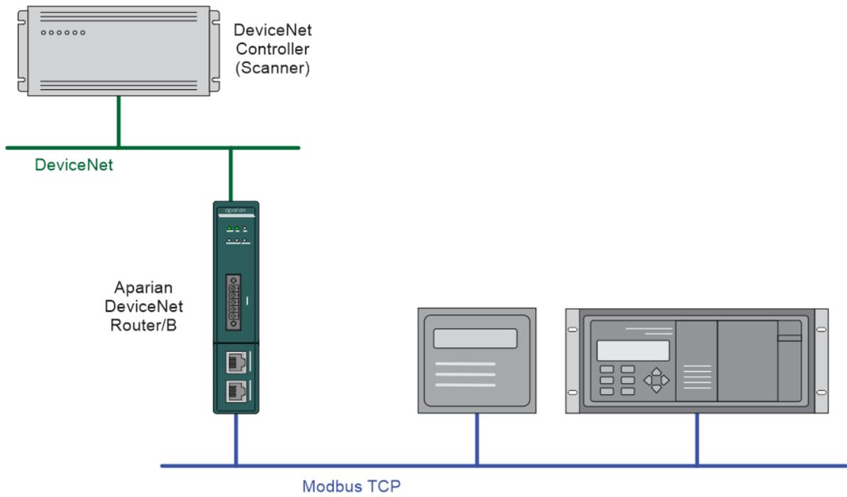
Figure 1.6. – Modbus TCP Device (Client or Server) operating as a DeviceNet Device
