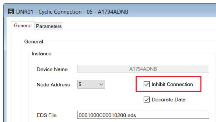
Figure 3.53 – DeviceNet Flex IO Adapter - Inhibit Connection
