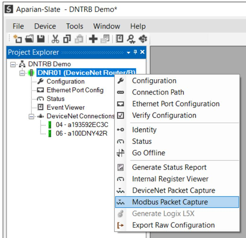
Figure 6.32 - Selecting Modbus Packet Capture
