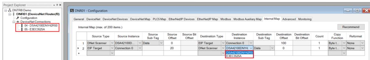
Figure 3.149 – IDS Copy – DeviceNet Scanner Destination Instance
