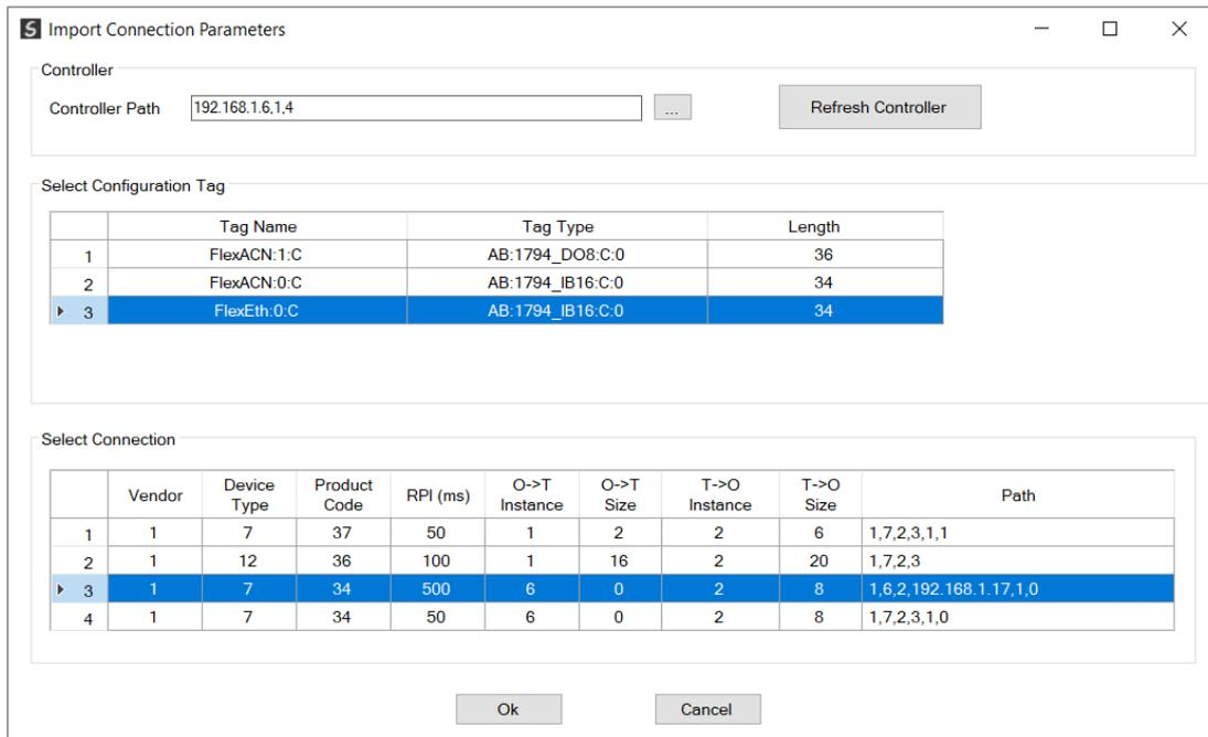
Figure 3.111 – Import Connection Parameters – Select Connection
