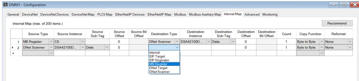
Figure 3.145 – IDS Copy - Modbus Destination Type
