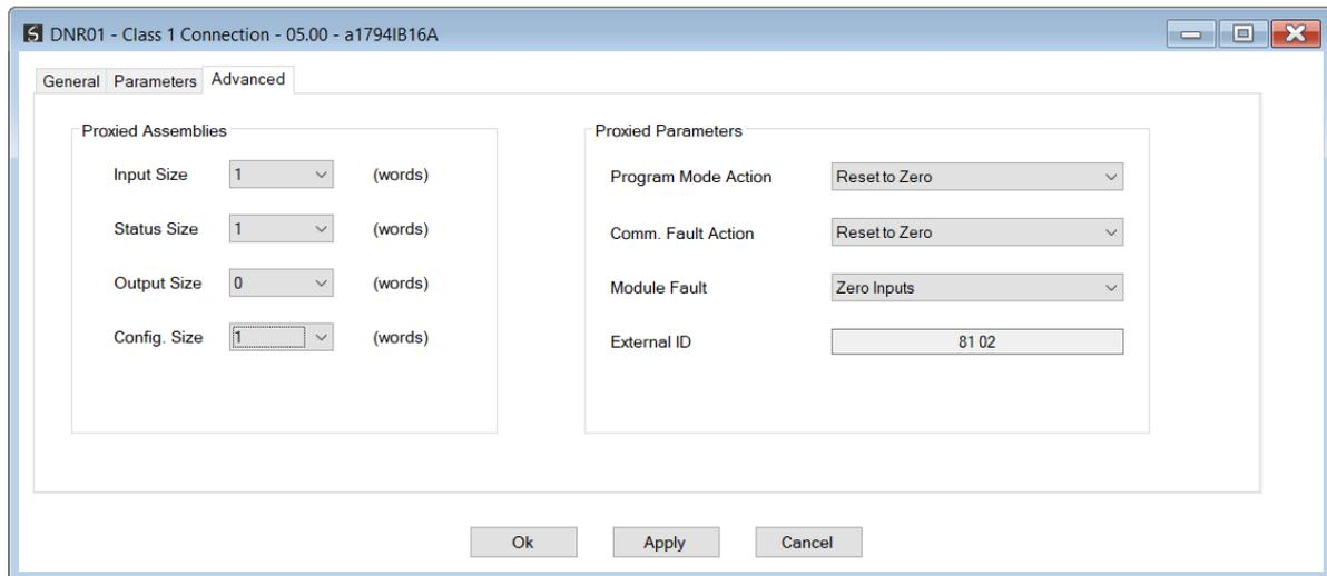
Figure 3.51 – DeviceNet Flex IO Module Advanced configuration
