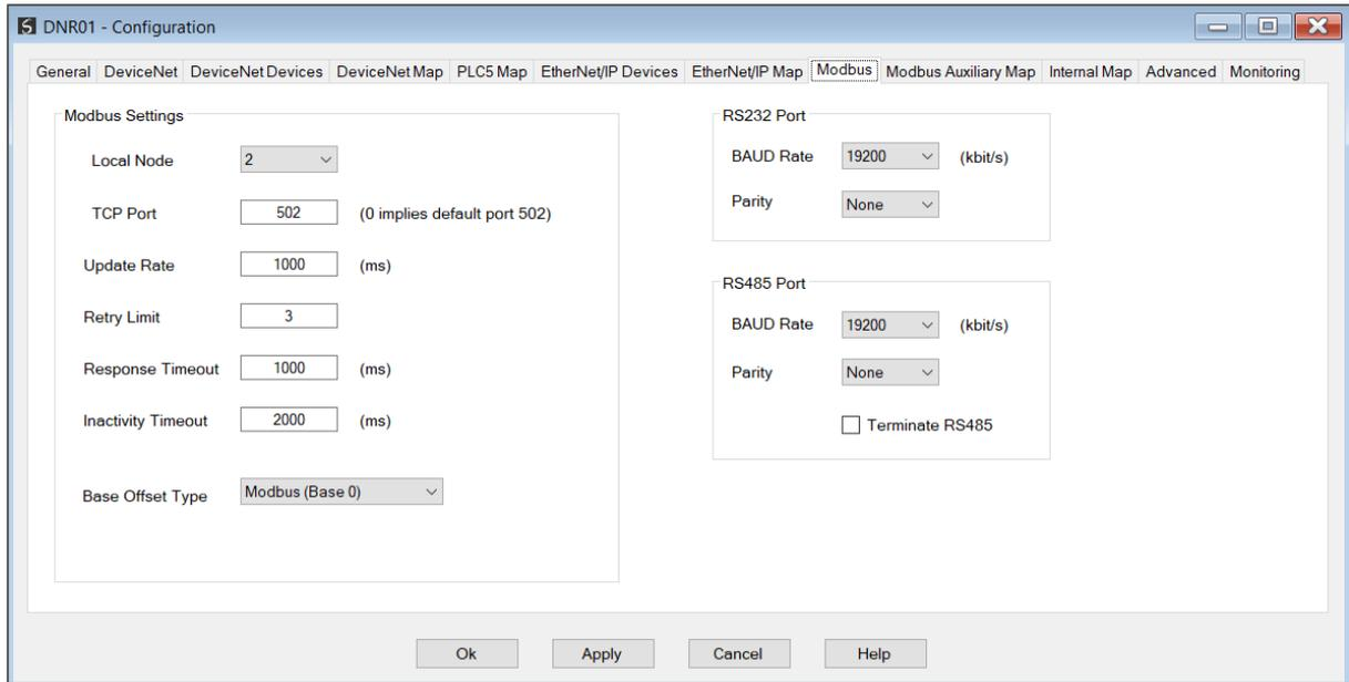
Figure 3.99 – Modbus Configuration
