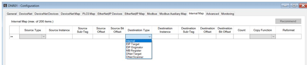
Figure 3.141 – IDS Copy – Internal Source Type
