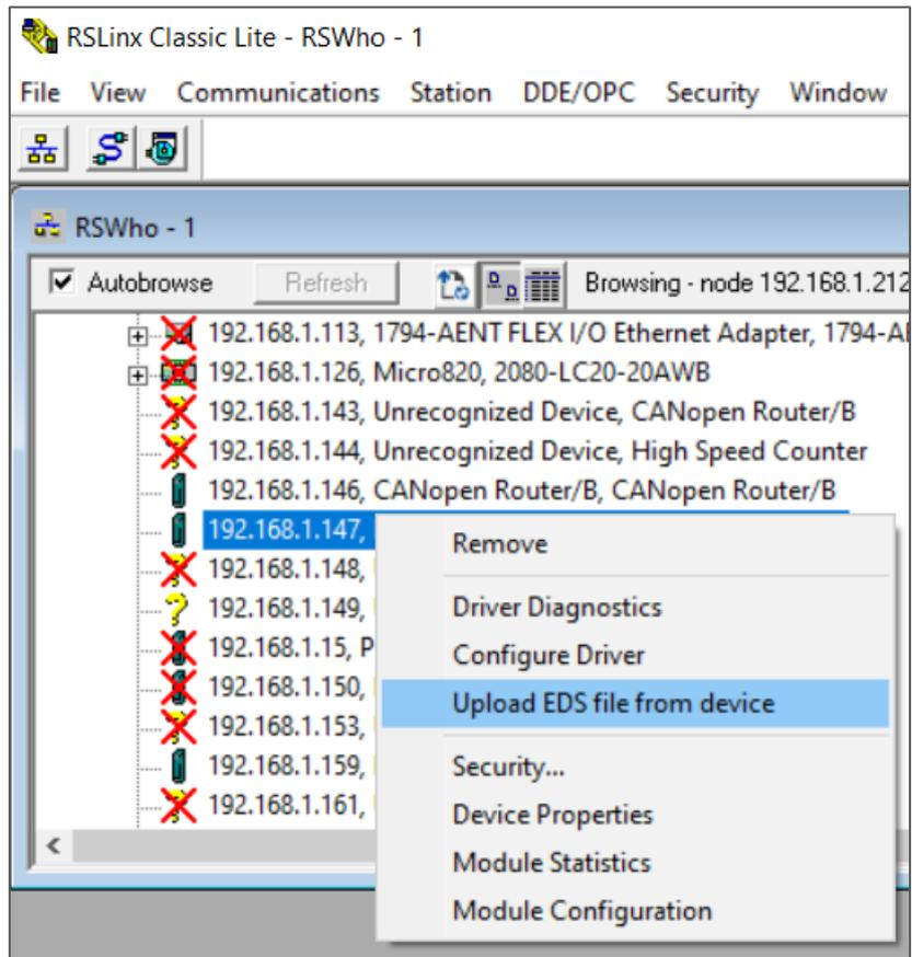
Figure 3.72 – EDS file upload from DeviceNet Router/B
