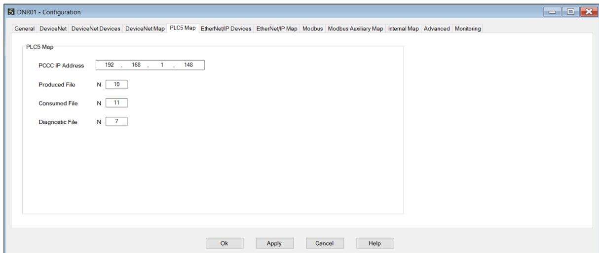
Figure 3.62 – PCCC Client Mode – IP Address Configuration
