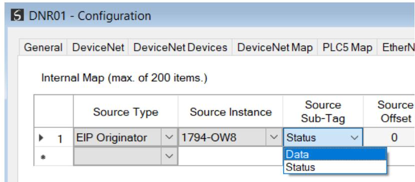
Figure 3.124 – IDS Copy – EtherNet/IP Originator Status
