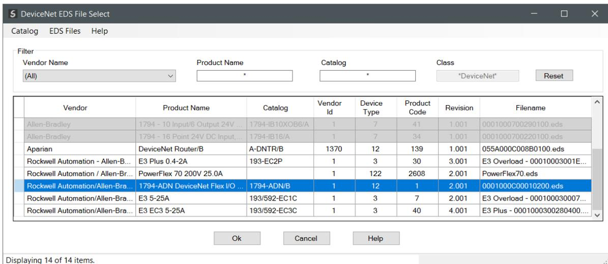
Figure 3.46 – Select the DeviceNet Flex I/O Adapter
