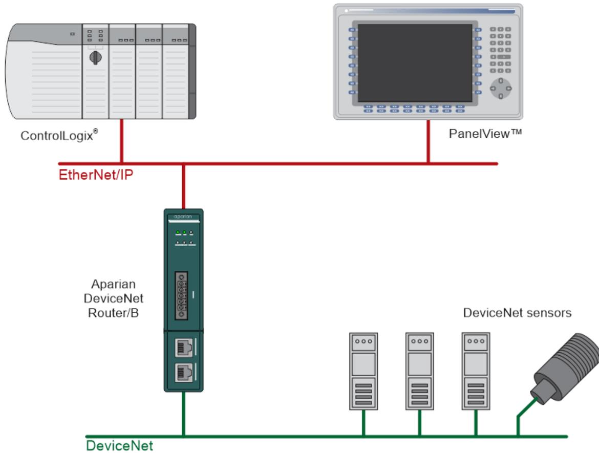
Figure 1.3. – Example of connecting DeviceNet Devices to a Logix Controller
