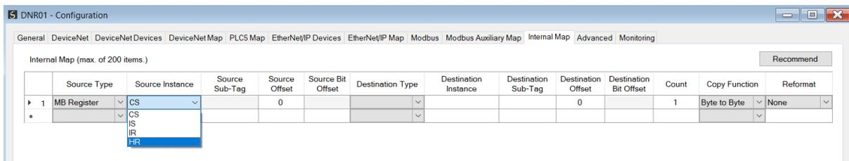
Figure 3.104 – IDS Copy - Modbus Source Instance
