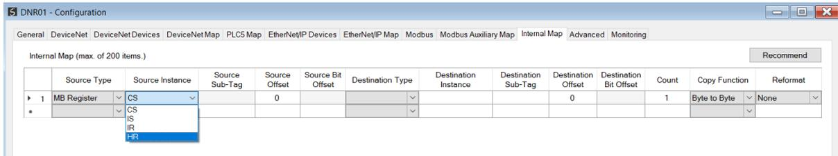
Figure 3.134 – IDS Copy - Modbus Source Instance
