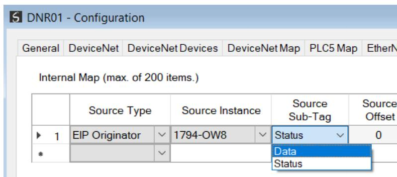
Figure 5.36 – IDS Copy – EtherNet/IP Originator Status
