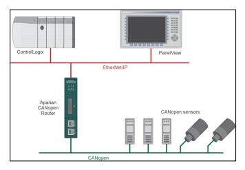
Figure 1 - CANopen Router with a Logix Controller
