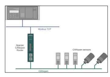
Figure 2 - CANopen Slaves to a Modbus TCP/IP Client
