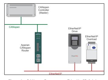
Figure 3 - CANopen Router as an EtherNet/IP Originator
