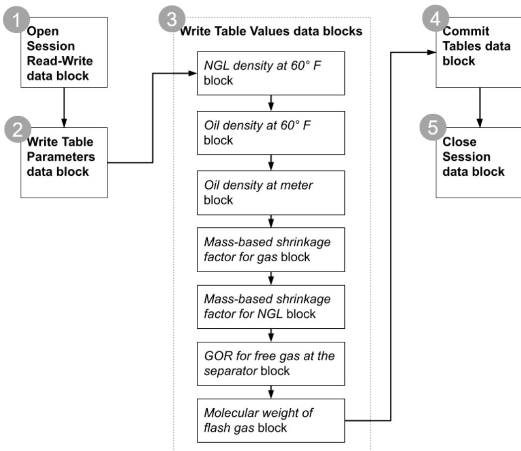
Sections 5.1.2 through 5.1.6 provide examples of the Modbus commands and data blocks that would be used to configure the example EOS table shown above.
