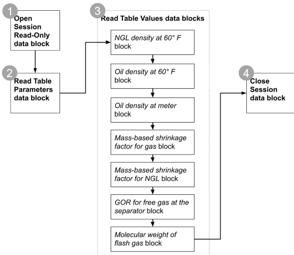
Sections 5.2.2 through 5.2.5 provide examples of the Modbus commands and data blocks that would be used to read the example EOS table shown above.
