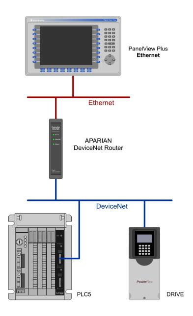
Figure 1 - Example of a typical network setup in PLC Emulation mode
