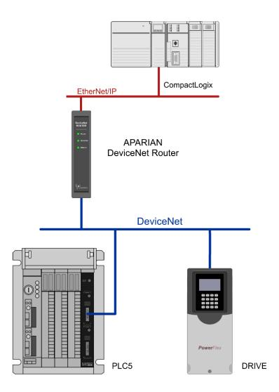
Figure 2 - Example of a typical network setup in Scheduled Parameter Mode
