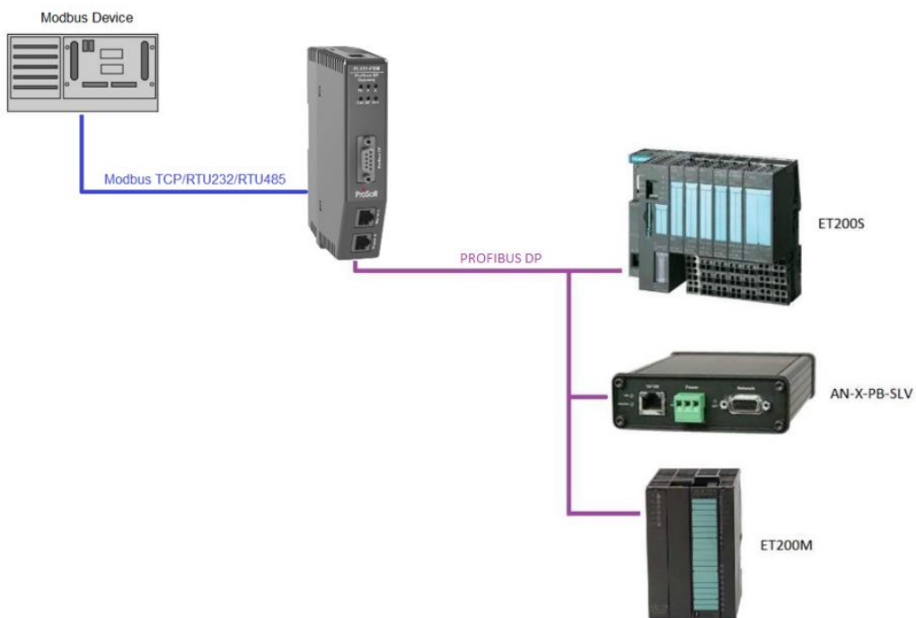
Figure 1.4 – PLX51-PBM PROFIBUS Master to Modbus (TCP/RTU232/RTU485) architecture
