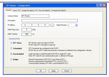
6. Click on the dotted button \_\_\_\_ to browse the PLX51 module in the **IP Address** section then you can select the module in the **Target Browser** window. Click on **OK** button.
