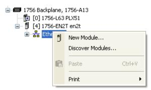
3. In the **Select Module Type** window select a **PLX51-DF1-ENI** module if you already have installed the EDS file if not, you can select a **Generic Ethernet Module**.
