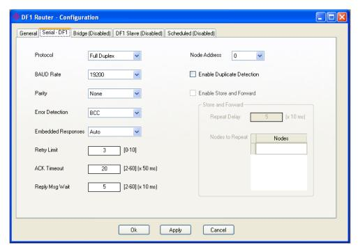
2. Configure the Message instruction, considering the configuration of each command in the MVI56-DFCM module.
