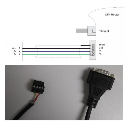
This is the pinout of the cable to communicate with PLC5.
