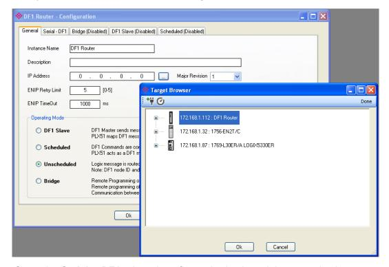
7. Go to the **Serial – DF1** tab and configure the basic serial communication parameter to match with PLC5 Chanel 0 configuration (see section III in this document).
