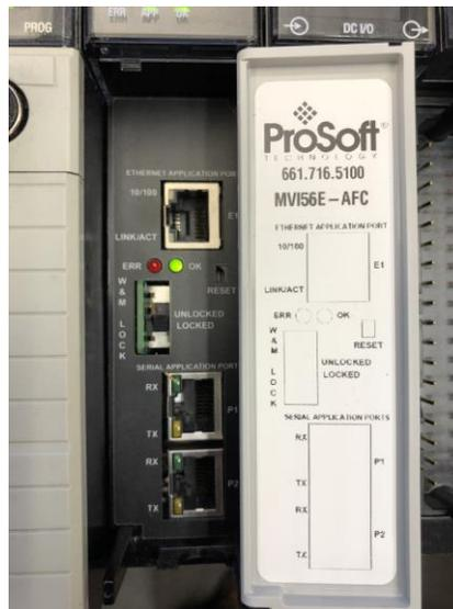
W&M lock switch in locked position with seal:
