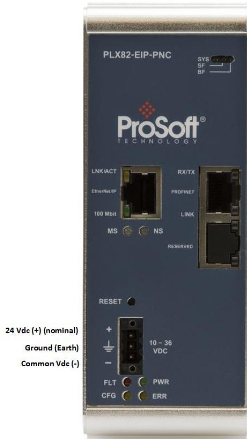
Use the J180 Power Connector to connect to the proper signals.
