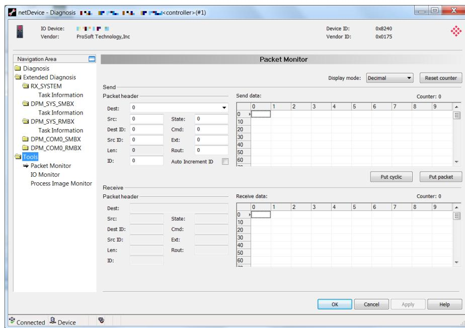
**DISPLAY MODE** switches the representation of data between decimal and hexadecimal.
