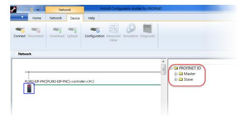
4 Open the device folder to display the device icon(s).
