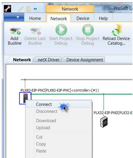
3 The module information located above the icon is highlighted in green once the connection is established.
