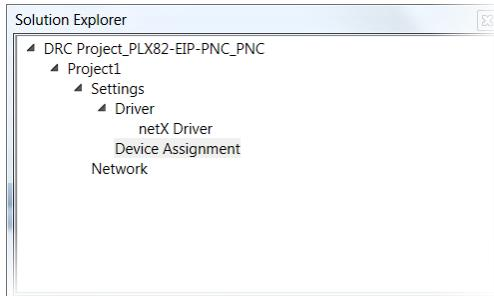
**2** Click on the **DEVICE ASSIGNMENT** tab and then click **SCAN**. The system scans for all devices that can be connected to the ProSoft fdt Configuration Manager software.
