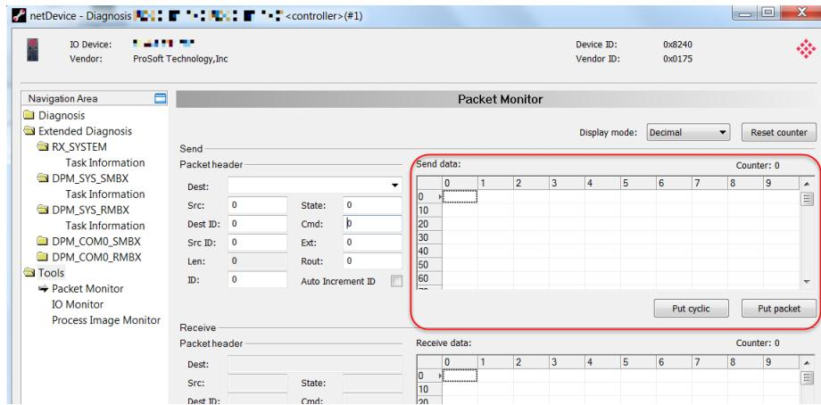
This area allows you to enter the send data of the packet that is transmitted from the application (configuration software) to the mailbox of the device. The description of the transmitted data depends on the command or response code.
