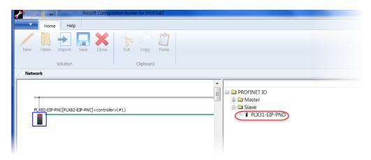
2 Drag and drop the slave onto the PROFINET bus line.
