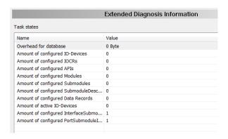
The T\_PNIO\_APCFG Extended Diagnostics Information displays PROFINET I/O specific parameters.
