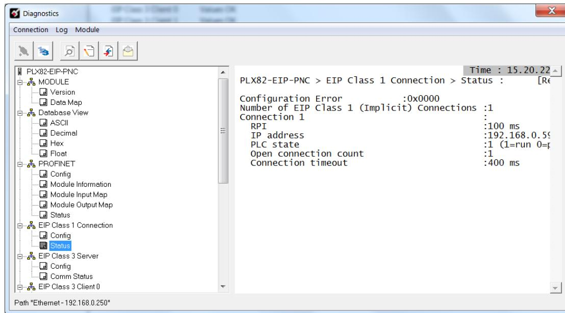
You can change the RPI and Ethernet IP in the ladder configuration in RSLogix 5000 (right-click **CONNECTION1** and choose **PROPERTIES**).
