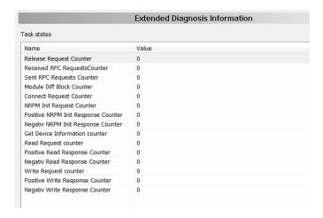
The T\_PNIO\_CMCTL Extended Diagnostics Information displays PROFINET I/O specific counters.
