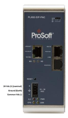
Use the J180 Power Connector to connect to the proper signals.
