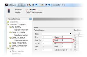
The **AUTO INCREMENT ID** checkbox specifies that the identifier should be incremented by one for each newly sent packet.
