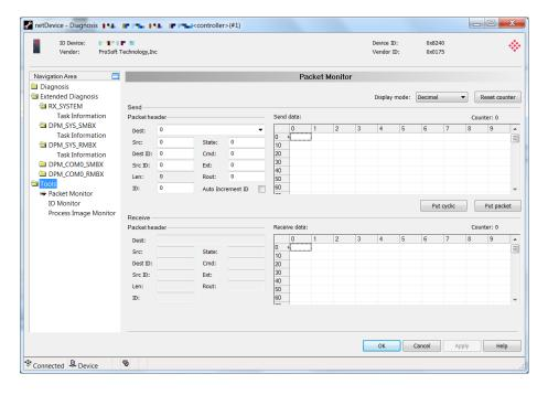
**DISPLAY MODE** switches the representation of data between decimal and hexadecimal. Use the **RESET** button to reset the packet counter.
