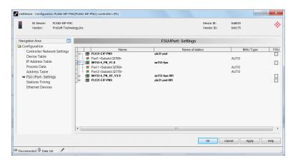
2 Check the **FSU** box for PROFINET devices that must use a fast startup (FSU) connection to establish cyclic data exchange.
