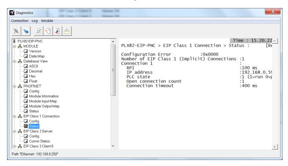
You can change the RPI and Ethernet IP in the ladder configuration in RSLogix 5000 (right-click **CONNECTION**1 and choose **PROPERTIES**).
