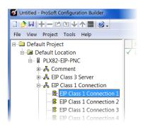
2 Double-click the **EIP CLASS 1 CONNECTION [X]** to display the *Edit - EIP Class 1 Connection [x]* dialog box.
