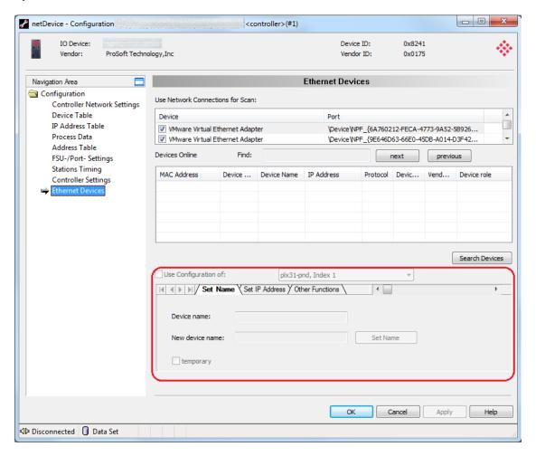
**Note:** If you are going to use a configuration from a different device, use the "Use Configuration of" section.
