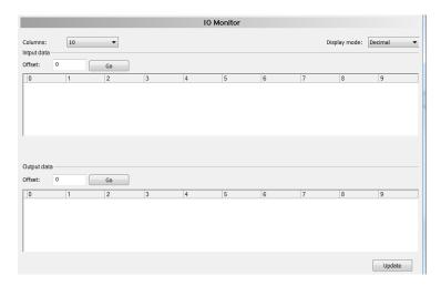
**Warning:** Only change and write output data if you know that it will not cause plant disturbances. All output data written by the I/O Monitor are transmitted at the bus and have an effect on subordinate drives, IO, etc.
