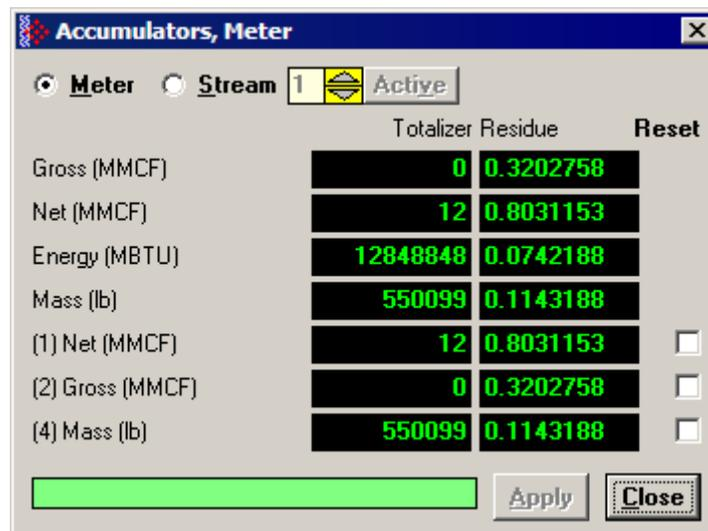
The total resettable accumulator 1 value (net) is 12.8031153.
