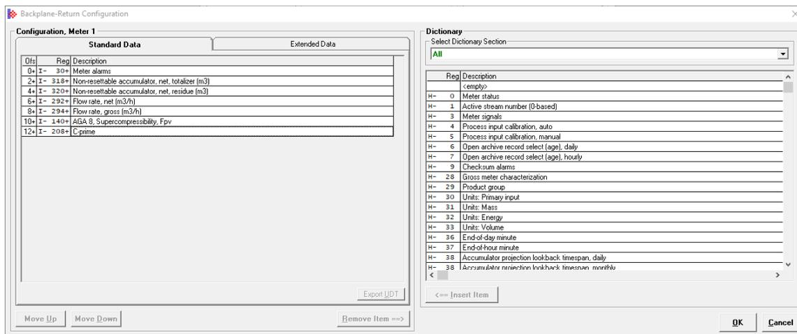
This example shows data that can be obtained via the *BackPlaneReturn.ProcessInput* tags of a meter tag structure. Once imported, the same data can be accessible from the PLC as shown:
