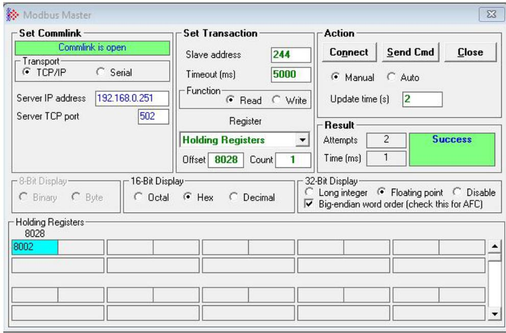
The hexadecimal value of the register is 8002, which is 1000 0000 0000 0010 in binary. The *Meter-group relationship* data point (position 15) has a value of 1, indicating that the meter has a relationship to a meter group. The *Group-parent meter channel* data point (positions 10 – 14) has a value of 0, indicating that Meter 1 is the parent of the group.
