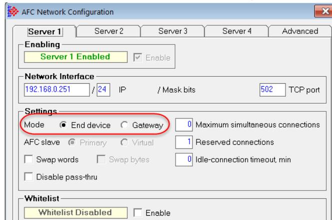
If set to an *End Device* (has its own Modbus database), the unit code is ignored and is echoed verbatim in the response regardless of its value.
