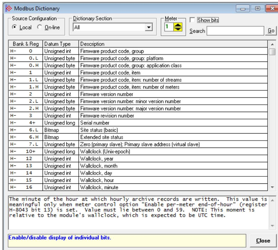
You can use the Modbus Dictionary locally or while EAFC Manager is directly connected to the module.
