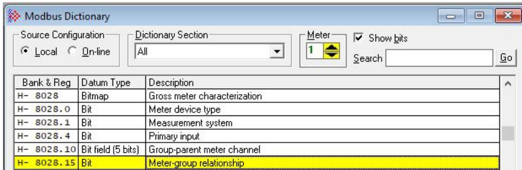
If Meter 1 is configured as a meter-group parent, we can use the Modbus Master dialog to poll the meter and obtain the value for holding register 8028, as shown in the following screen capture:
