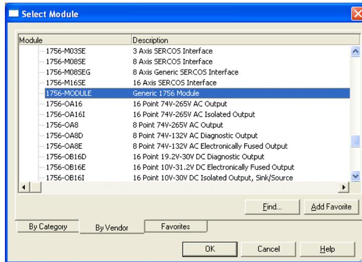
6 Create a new **1756-MODULE** (I/O Configuration) with the following settings:
