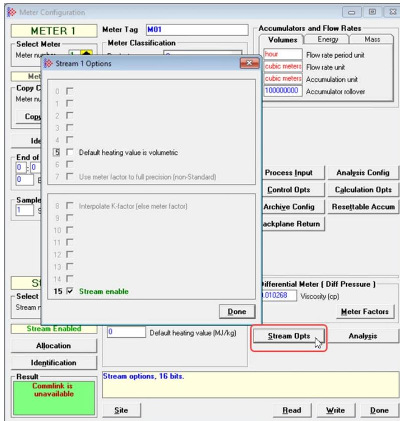
A meter has one active stream which corresponds to the particular product that flows through the meter at that moment.
