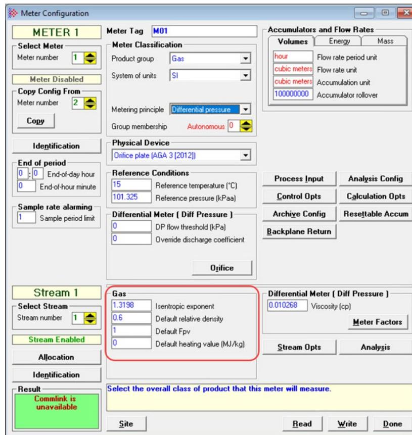
The *Gas* area of the *Meter Configuration* dialog is visible when the product group is set to *Gas*.
