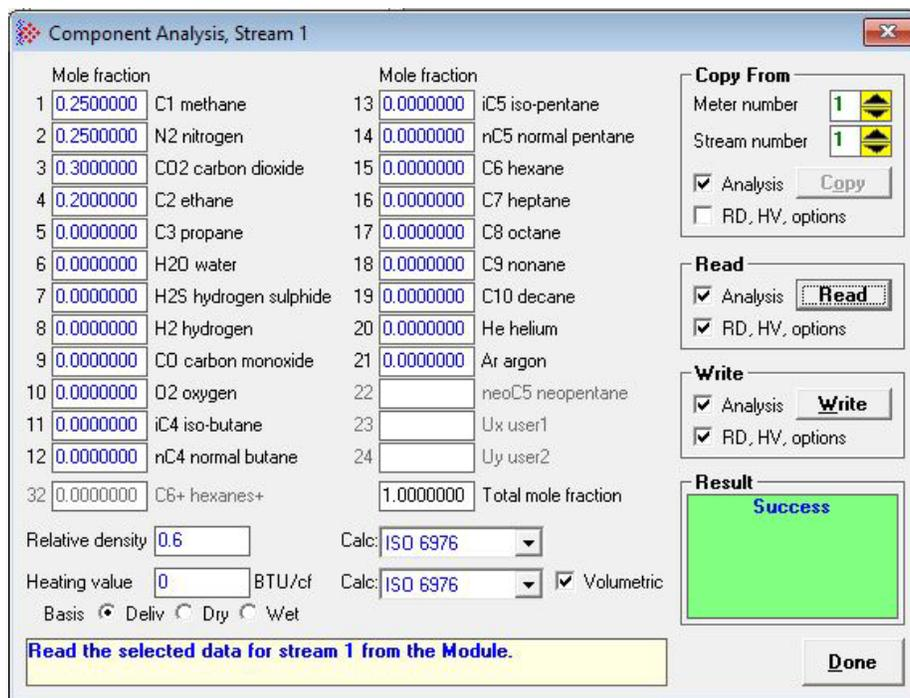
The *Component Analysis* dialog box for a member of the parent’s group would look like the following screen capture. Note that many of the parameters are disabled (grayed out). That is because the values for these parameters are sourced from the meter-group parent.
