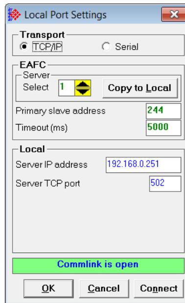
Adjust the communication settings if necessary. Click **CONNECT** to save the settings and **OK** to connect.
