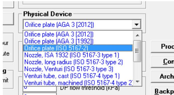
If you are using a differential gas type principle, measuring differential pressure, you have the option of selecting from the following standards:
