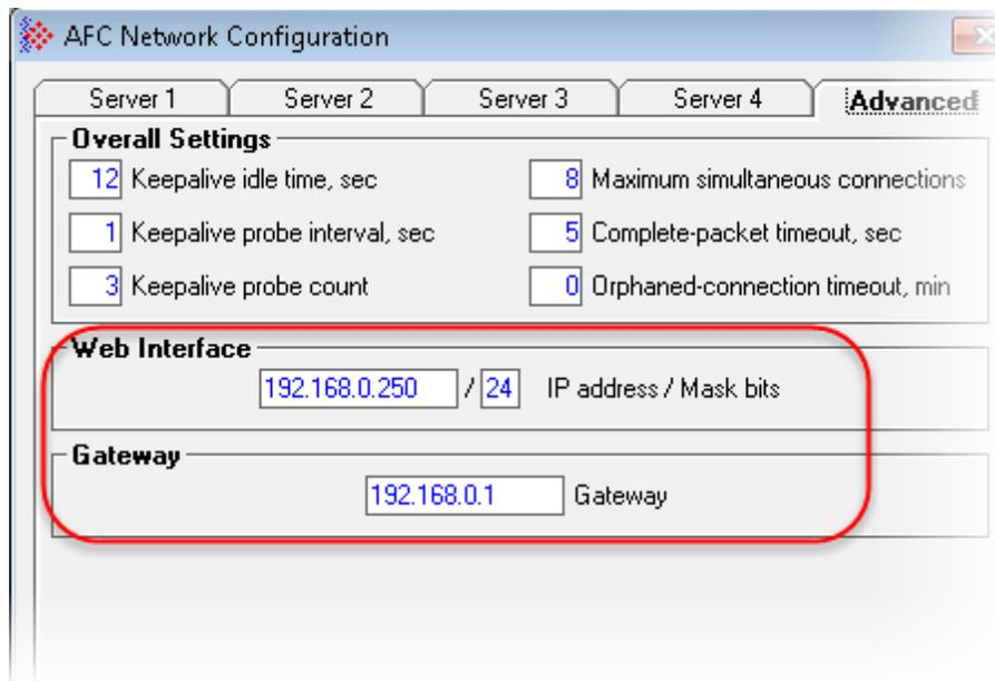
The IP address and Mask bits pertain to the address of the AFC module. This is not a Modbus TCP/IP address used by the AFC module. The default web interface address is 192.168.0.250.
