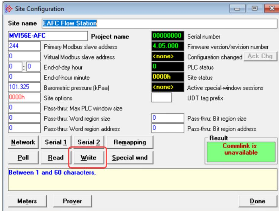
After writing the configuration to the module, you can click the **READ** button to read the current module site configuration. The configuration should match the last write operation data.
