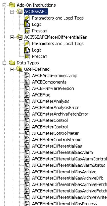
The procedure has imported controller tags that will be used by the sample program.
