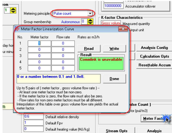
Meters may begin to wear out over time and the actual measured volume (the "gross volume") will tend to drift from the nominal measured volume (the "indicated volume"). The factor that corrects "indicated" to "gross" is called the "meter factor", and is a number very close to 1.
