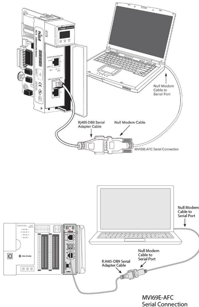
The null-modem cable that is supplied with the module uses the following cabling scheme:
