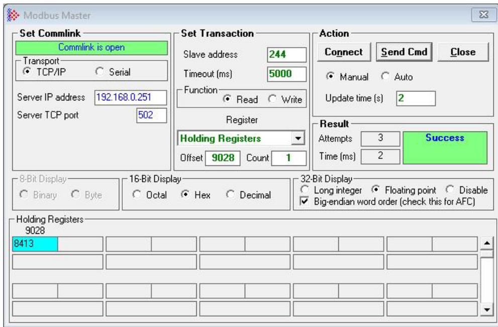
In this example the hexadecimal value of the register is 8413, which is 1000 0100 0001 0011 in binary. The *Meter-group relationship* data point (position 15) has a value of 1, indicating that the meter has a relationship to a meter group. The *Group-parent meter channel* data point (positions 10 – 14) has a value of 1, indicating that Meter 2 is a member of the group having Meter 1 as its parent.
