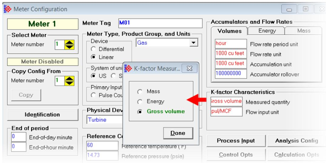
Click the *Flow input unit* field to choose the flow input unit for this meter.
