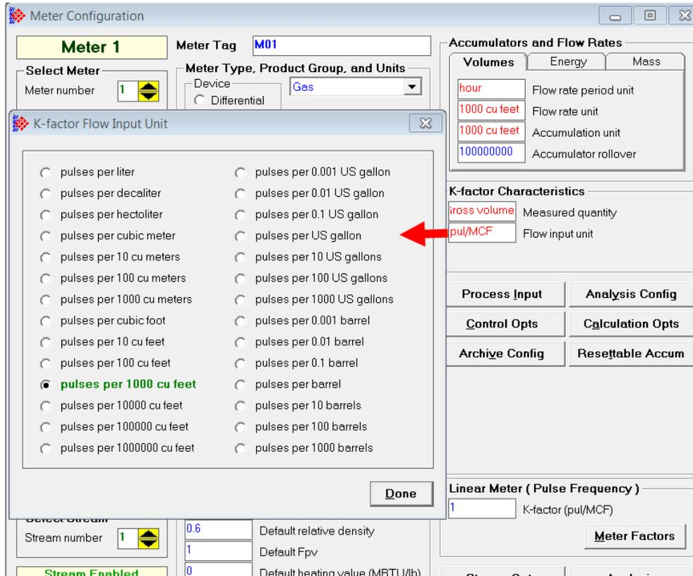
The K-factor itself is entered as a stream parameter. The K-factor units available for selection will depend on the selected measured quantity.
