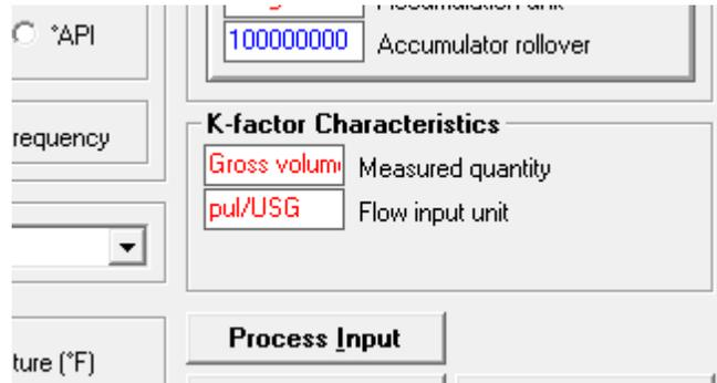
The *K-factor Characteristics* area of the *Meter Configuration* dialog is visible when the metering principle is either *Pulse Frequency* or *Pulse Count*.
