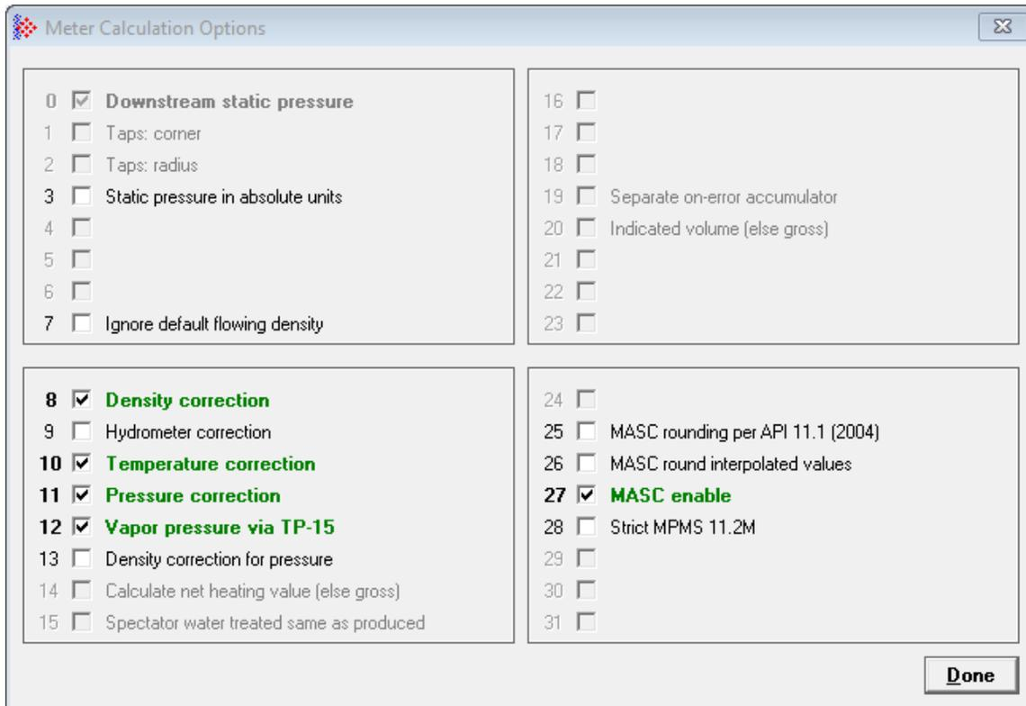
Options that do not apply to the current application are grayed out. See “Meter Calculation Options” in the *AFC Reference Guide* for detailed information.
