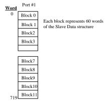
The following diagram shows the Slave #1 Data block broken down into its 60 word blocks, and the corresponding BTR Block ID number for each of the blocks.
