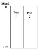
In order to get this data into the PLC/SLC, the blocks are broken down into 60 word 'pages' and transferred to the ladder logic across the backplane using the standard BTR or M1 instructions. The following sections detail the structure of this data and the mechanism by which all of the data is transferred.
