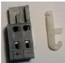
The Power Connector (ProSoft part number 002-0116) is shown on the left. Note the + and – polarity markings. The connector lever (ProSoft part number 357-0061) shown on the right is helpful for installing wires into the spring-loaded contacts inside power connector.
