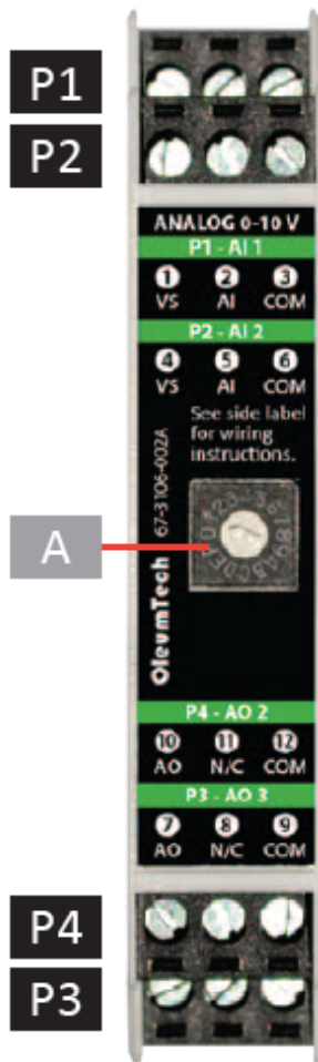
A - 16-Position ID Switch For Matching Module ID
