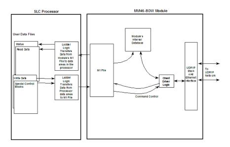
All data transferred between the module and the processor over the backplane is through the M1 file. Ladder logic must be written in the SLC processor to interface the M1 file data in the module's internal database. All data used by the module is stored in its internal database. This database is defined as a virtual data table with addresses from 0 (40001) to 4999 (45000). The following illustration shows the layout of the database:
