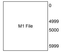
Data registers in the module above 4999 are used for command control. When special values are written in this register set, the module will perform specific functions. The following topics define the special functions handled by the module.
