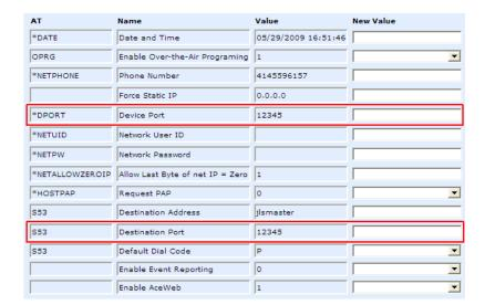
The destination port for the modem at the host needs to match the device port in use on all the modems at the remote sites. For example, if the remote modem's device port (see below) is "12345", then the Modbus host modem's **\$53** destination port should be set to "12345".
