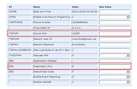
The destination port for the modem at the host needs to match the device port (\*DPORT) in use on all the modems at the remote sites. For example, if the remote modem's device port (\*DPORT) is "12345", then the Modbus host modem's \$\instyle{5}3\$ destination port should be set to "12345".
