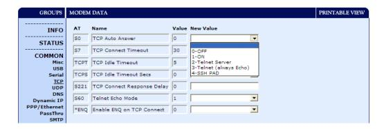
If you need to change the port for Telnet (for example, you have the default port blocked on your firewall), the option is on the **OTHER** tab. The default telnet port is 2332. You can also change the Telnet timeout, if the connection is idle, default 2 minutes.
