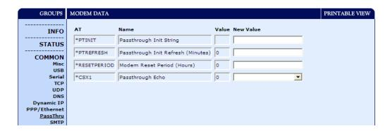
PassThru Mode allows only specific AT commands. Some ALEOS commands will be unavailable when the RLXIC-SG is in PassThru mode. The commands usable also depend heavily on the modem model number (found on the label on the top of the RLXIC-SG).
