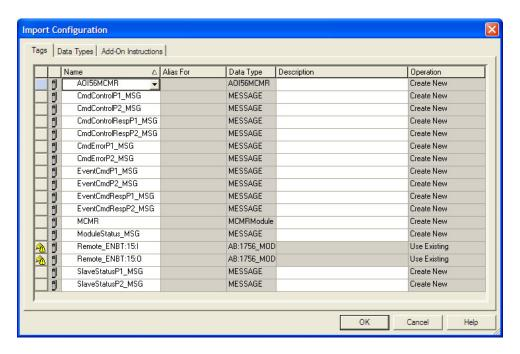
15 If you are using the module in a different slot (or remote rack), select the correct connection input and output variables that define the path to the module. If your module is located in Slot 1 of the local rack, this step is not required.
