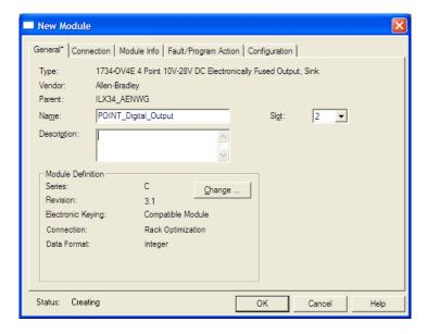
In the **Module Definition** area of the dialog box, notice that the default Connection type is **RACK OPTIMIZATION**.
