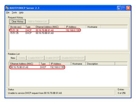
To assign this configuration to the device, select the device in the **RELATION LIST** pane, and then click the **DISABLE BOOTP/DHCP** button. The device will use the assigned configuration the next time it is powered up, and will no longer issue DHCP requests.
