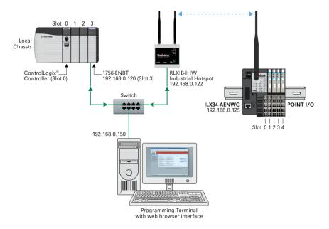
**Note:** During the installation, you must connect to the ILX34-AENWG directly via Ethernet to set its wireless settings so it can communicate with its Access Point. To prevent a loop from occurring, avoid connecting Ethernet cables to the Access Point and the ILX34-AENWG at the same time after the wireless link is established.
