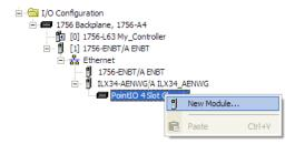
2 In the SELECT MODULE dialog box, choose the 1734-OW2 relay output module from the list, and click OK.
