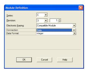
4 Click the CONNECTION tab, and then change the RPI value for the module from 20 (the default) to 50 (the recommended value for analog or specialty modules). This value determines how often to exchange data with the ILX34-AENWG adapter.
