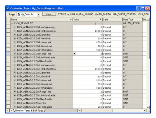
5 Click the value 2 and change it to 0, which changes the voltage range to -10 to +10V dc for channel 0.
