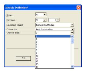
2 Select the Chassis Size for your project from the dropdown list, and then Click **OK** to close the **Module Definition** dialog box. In a later step, you will verify the chassis size when you are online with the Configure 1734 POINT I/O Modules (page 40).
