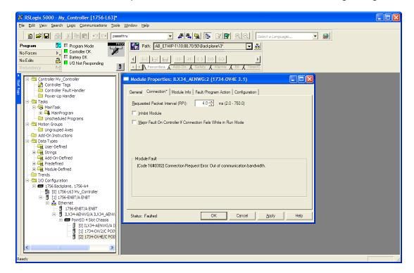
If you encounter this condition, the only action you can take is to alter the existing connections to reduce the amount of microprocessor bandwidth consumed. The most likely fixes for this condition include the following.
