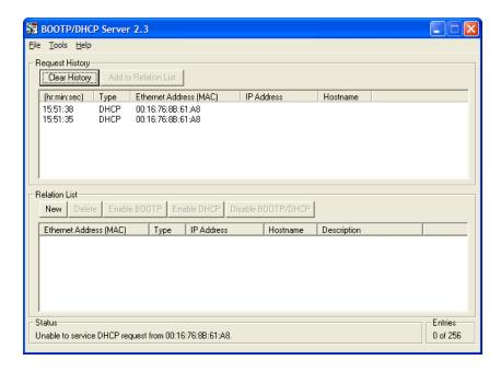
2 Double-click the hardware address of the device to configure. This action opens the NEW ENTRY dialog bow, populated with the device's Ethernet Address (MAC).
