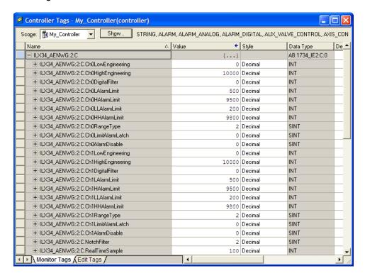
2 Expand the configuration tag ILX34 AENWG:2:C.
