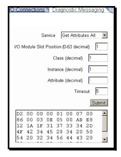
The data is returned in hexadecimal format. Refer to the documentation for each POINT I/O Additional Point I/O Documentation (page 170) to determine the meaning of the response.
