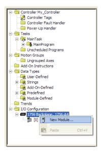
2 Expand the **COMMUNICATIONS** node, and then select the **ETHERNET BRIDGE** module that matches your hardware. This example uses a 1756-ENBT/A module.
