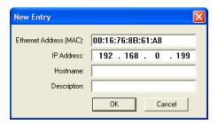
3 Enter the IP Address to assign to the device, and click **OK.** You can leave the **HOSTNAME** and **DESCRIPTION** fields blank.
