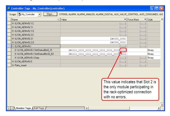
Use the controller tags in your ladder program to read input data or write output data.
