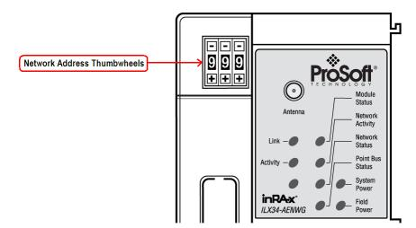
The three thumbwheel switches represent the final octet for the private IP address 192.168.1.xxx (where xxx represents the number set on the switches).
