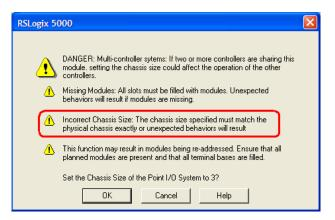
**6** Notice the chassis size in the module has been updated to match the hardware configuration.
