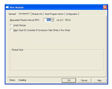
**Important**: To avoid overloading the ILX34-AENWG adapter, we recommend that RPI be no less than 10 ms for rack connections and 50 ms for direct connections.
