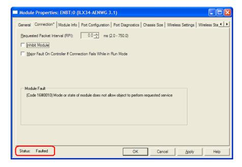
The module is faulted because, even though you set up the adapter's POINT I/O chassis size to the actual number of modules, plus the adapter, the adapter still remembers the size of 1 (the factory default value) until you reset this size manually.
