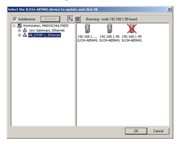
Any ILX34 devices detected will appear in the right pane as in the above example. For our example, we will flash the device shown at IP address 192.168.1.90. (Note that the device at 192.168.1.99 was detected in a previous ControlFLASH session, but it can be ignored.)
