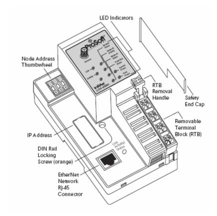
The Wireless POINT I/O Adapter is a communications adapter for POINT I/O modules. The adapter provides an interface for controlling and communicating with POINT I/O modules from an Ethernet network.
